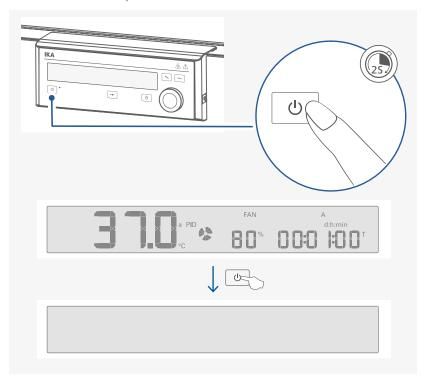
**Note:** When switching the device to standby status, if the device chamber temperature is higher than 50 °C, the actual temperature is displayed, e.g. 70 °C and "hot" symbol blinks.
