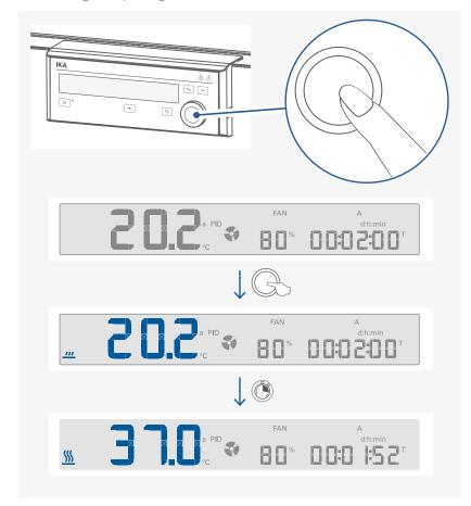
**Note**: At set temperatures below the ambient temperature, the cooling unit switches on automatically. Please note that ice may form in the interior during cooling mode.
