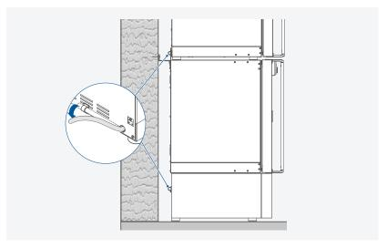
Extend the drain hose as required using the enclosed hose adapter
