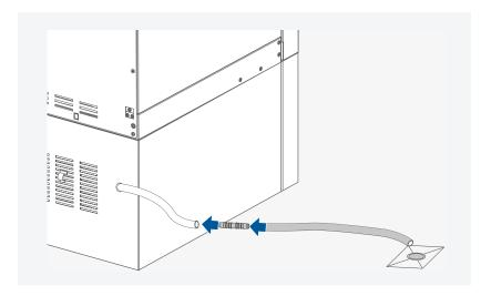
Water caused by condensation or defrosting is directed into the drain hose at the rear of the device. Place the drain hose in the laboratory drain.
