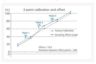
Individual load and ambient condition might influence the temperature behaviour of the chamber. To compensate that influence there's the option to neutralize by using the 3-point calibration and offset function. This function allows the temperature to be calibrated and adjusted at three different temperature values.
