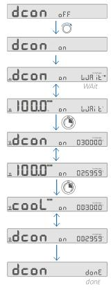
When the decontamination process is finished, the "dcon donE" appear on the display and a "beep" sound is heard.
