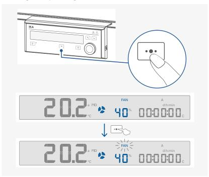
**Note:** Press the multifunction key (F) to activate the fan speed setting. The fan symbol blinks. Then, the fan speed value can be adjusted by rotating the control knob (H).
