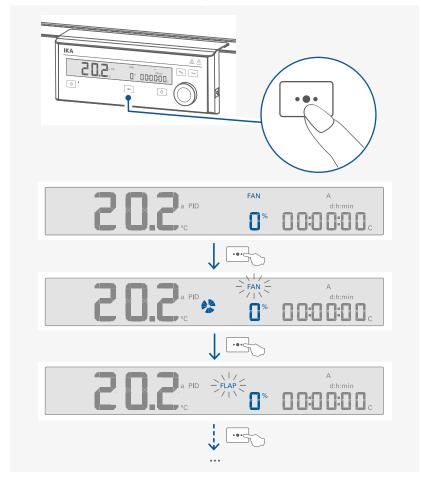
**Note:** Press the multifunction key (F) to switch between the settings for the fan and the ventilation flap. The selected function blinks. Then, the value can be adjusted respectively by rotating the control knob (H).
