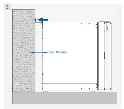
**Note:** The screws used for fixing is selected according to the wall conditions and is not included.
