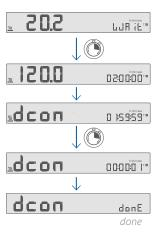
When the decontamination process is finished, the "dcon done" appear on the display. Press control knob to confirm it and screen back to "dcon off" as below:
