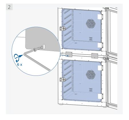
> Fix the top device to the wall
