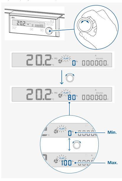
**Note:** The ventilation flap value can also be changed when the heating function is activated.
