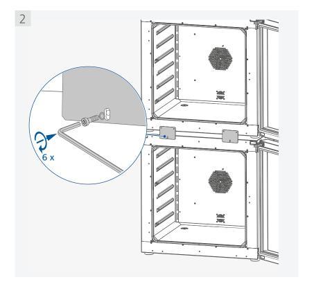
> Fixing the top device to the wall
