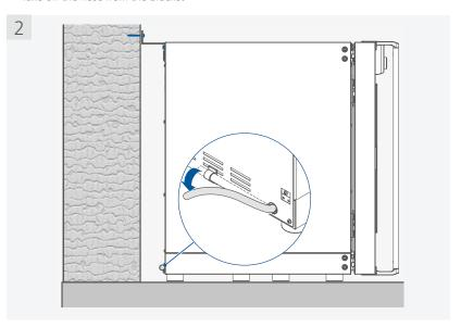
> Extend the drain hose with included hose adapter as necessary
