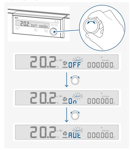
**Note:** When the device is running, the light status can also be changed.
