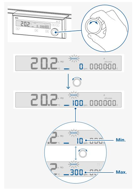
**Note:** When the device is running, the shaker speed can also be adjusted.
