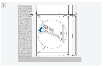
Extend the drain hose with included hose adapter as necessary
