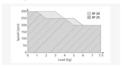
In order to ensure safe and secure operation, the shaker platform must only be operated within the range of usable weight and speed (see diagram - hatched area).
