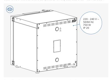
**Note:** The voltage stated on the type plate must correspond to the power voltage.
