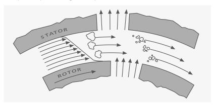
The dispersion effectiveness is heavily dependent on the product of the shear gradient and the time the particles spend in the shear zone. The optimum range for the circumferential velocity of the rotor / stator arrangement is 6-24 m/s.
