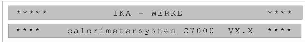
The letters VX.X give the software version installed in the instrument.
