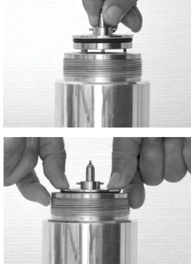
Place the union nut onto the lower section and tighten by hand.
