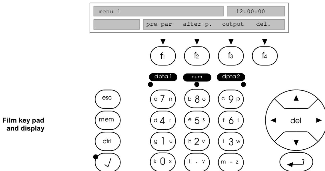
1. **Function buttons *f1*, *f2*, *f3*, *f4***: The functions of the buttons *f1*, *f2*, *f3*, *f4* are always indicated by the text that appears in the lower right zone of the LCD display. The relevant text in the display is directly above its button:
