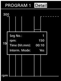
Turn the rotary/push knob, the details screen of every segment can be switched.
