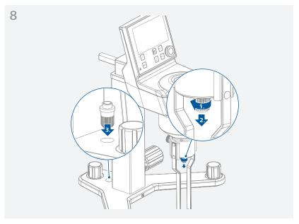
**Note:** The protection cap protects the coupling nut and the inside pivot from damage during transportation. Keep the protection cap in the hole of the stand in order to avoid missing!
