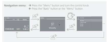
**Note:** If you press the "Menu" key, the system skips directly back to the working screen. If you press the "Back" key, the system skips back to the previous display.
