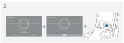
**Note:** The short horizontal white line inside the circle is moving vertically and it represents the rotation around the Y-axis. When it matches the white line, the device will be in balance with the Y-axis, then the line color will turn from white to green.
