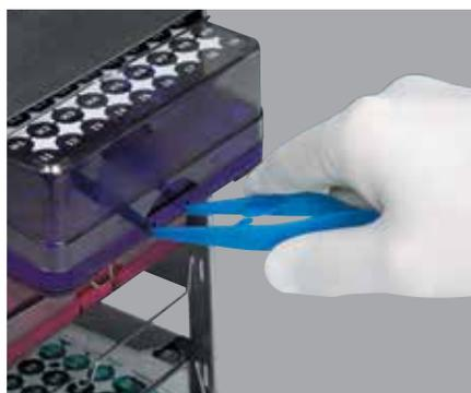
Forceps included with boxes b, d, can be used to pick vials or remove box from freezer rack
