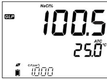
The cell factor in cm<sup>-1</sup> determined from the calibration with the current reading.
