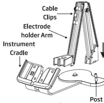
Slide edge<sup>EC</sup>® into the cradle while positioning the probe cable behind the cradle. Put the probe/sensor into the electrode holder and secure cable in clips.
