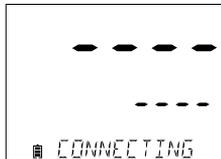
Connect the 3 mm probe jack to the probe input located on the bottom of edge<sup>EC</sup>®. **Make sure the probe is completely connected.** If the probe is recognized, "CONNECTING" message is displayed along with sensor model.
