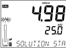
When the reading is stable and close to the selected standard, “CFM” tag will blink, the message “SOL STD” and the value will be displayed.
