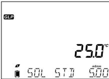
The Solution Standard and calibration temperature.
