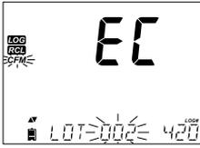
Connect USB flash drive to the USB port, located on the top of the meter. Press the RCL key. Press the CFM key. Select Manual, Stability, or interval lots by using the ▲▼ keys. Press the LOG key (not CFM). The "USB HOST" tag should come on.
