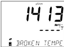
The Log file will indicate a “°C!” next to the data. In the case the temperature sensor is damaged, “BROKEN TEMPERATURE SENSOR” , “---” along with NoTC tag will be displayed and the unit tag will blink on the LCD. If logging when this occurs, the Log file will indicate “°C!!” next to the data. Absolute conductivity (NoTC) will be marked with an “A” in the CSV files and dashes will appear in the temperature field.
