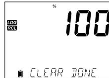
Logged data on edge<sup>EC</sup>® can be transferred from the meter to a USB flash drive by using the log recall function. The minimum requirement for the drive is USB 2.0. Select the EC record you wish to export and follow the simple steps below.
