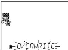
If the selected file is already saved on the flash drive, edge<sup>EC</sup>® will ask for confirmation of overwriting the existing file. The message "OVERWRITE" and "CFM" tag will blink. Press CFM for overwriting the existing file or CAL to exit without exporting.
