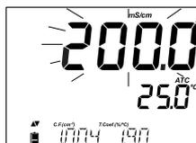
**Note:** Temperature-compensation and absolute conductivity (NoTC) are selected in the SETUP configuration.
