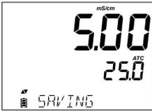
Press CFM to confirm calibration. The instrument displays “SAVING”, stores the calibration values and returns to measurement mode.
