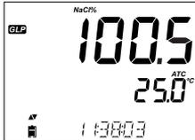
The time (hh:mm:ss) of the last calibration together with the current reading.
