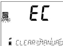
Select the Manual (Stability) lot and press CLR. The "CLEAR" message will be displayed along with "MANUAL" or "STABILITY" and CFM tag blinking on the LCD. Press the CFM key to confirm the deleting of the selected lot (MANUAL or STABILITY) or all records. Press CLR to exit without deleting.
