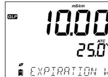
If enabled, the number of days until the calibration alarm "CAL DUE" will be displayed. (i.e. "CAL EXPIRES IN 2 DAYS")
