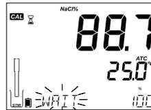
When the reading is stable and close to the standard, "CFM" tag will blink and "SOLUTION STANDARD" message will be displayed.
