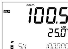
**Note:** Press GLP at any moment and the instrument will return to measurement mode.
