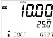
The salinity coefficient determined from the calibration together with the current reading.
