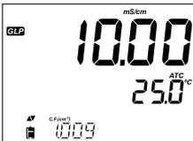
The cell factor in  $\text{cm}^{-1}$  determined from the calibration with the current reading.
