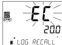
If no data was logged for the selected measurement range, the instrument displays the following messages:
