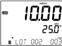
A "PLEASE WAIT" message will be displayed followed by the number of free spaces. During active interval logging, lot information is displayed on the third LCD line. The line indicates in which lot the data will be placed and keeps track of the number of logged records taken. The "LOG" tag is continuously on during active logging.
