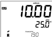
The temperature coefficient used during calibration with the current reading.
