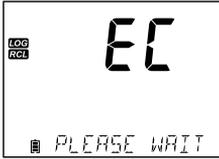
For Interval lots, the message "CLEAR", followed by the selected lot will be displayed with "CFM" tag blinking. Press the ▲▼ keys to select a different lot. Press CFM. The instrument will display "PLEASE WAIT".
