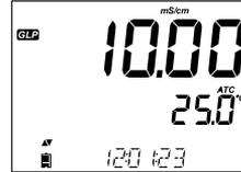
The date (yyyy.mm.dd) of the last calibration together with the current reading.
