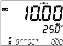
The calibration offset factor in  $\mu\text{S}/\text{cm}$  together with the current reading.
