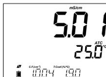
To toggle between information displayed on the third LCD line, use the ARROW keys.
