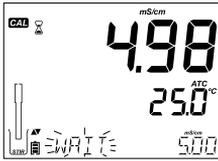
Press CAL to enter calibration. The “CAL” tag and the recognized standard value will appear on the third LCD line. If necessary, press the ARROW keys to select a different standard value. The “
