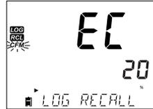
"CLEAR ALL" will be displayed with "CFM" and "EC" tags blinking. Press CFM.
