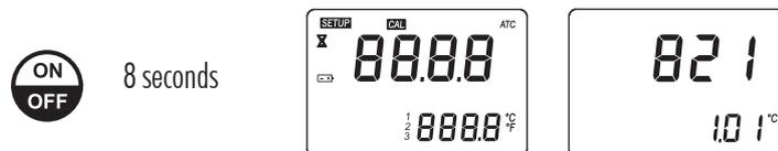
2. While continuing to hold the **ON/OFF** key, press the **ZERO** key. The temperature unit will change from °C to °F or vice versa.
