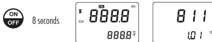
2. While continuing to hold the **ON/OFF** key, press the **ZERO** key. The temperature unit will change from °C to °F or vice versa.
