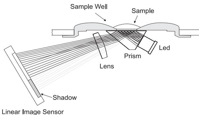
Specialized algorithms then apply temperature compensation to the measurement and convert this refractive index to the model specific measurement unit.
