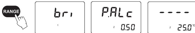
2. The potential alcohol scale also indicates the conversion factor chosen for the potential alcohol reading. See TO CHANGE POTENTIAL ALCOHOL CONVERSION FACTOR (page 13) to change the current factor.
