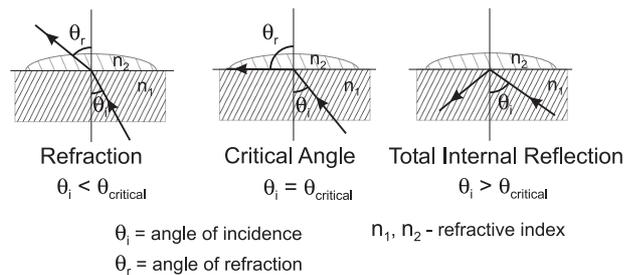
In the Hanna wine measurement refractometers, light from an LED passes through a prism in contact with the sample. An image sensor determines the critical angle at which the light is no longer refracted through the sample.
