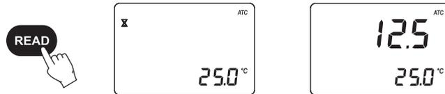
**Note:** The "ATC" tag blinks and automatic temperature compensation is disabled if the temperature exceeds the 10-40 °C / 50-104 °F range.
