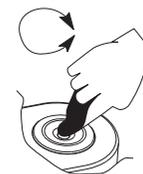
2. Using plastic pipettes, drip sample onto the prism surface. Fill the well completely.
