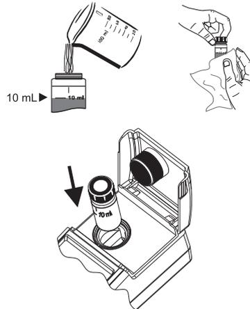
**Note:** If you have a cuvette with orientation mark place the cuvette with the orientation mark aligned with the sign on the instrument top.
