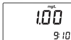
**Note:** The reading should be within specifications as reported on the CAL CHECK™ Standard Certificate. If the value is found out of specifications, please check that the cuvettes are free of fingerprints, oil or dirt and repeat validation. If results are still out of specifications, then recalibrate the instrument.
