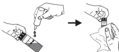
**Note:** The supplied cloth for oiling should be stored together with the silicone oil bottle and cuvettes, taking care to avoid contamination with dirt. After a few oiling procedures, the cloth will contain enough oil to wipe the bottle with it without adding more oil. From time to time add some drops of oil on the cuvette to provide the necessary oil quantity in the cloth.
