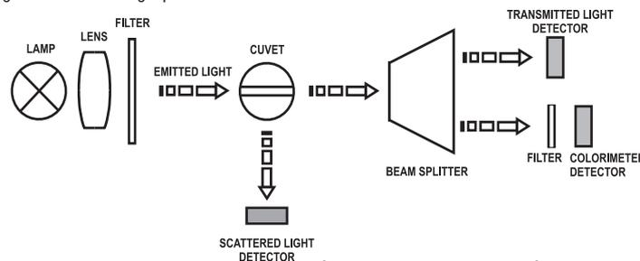
For the turbidimeter range the microprocessor of the instrument calculates from the signals that reaches the two detectors, the NTU value, using an effective algorithm. This algorithm corrects and compensates for interferences of color, making the **HI 93414** instrument color-compensated.
