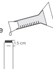
Insert the reacted sample into the cuvet holder and make sure that the notch on the cap is positioned securely into the groove. Wait 30" and then press READ.
