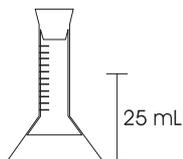
Add the content of one packet of **HI 93746** TPTZ reagent, close the cylinder and agitate for 30 seconds.
