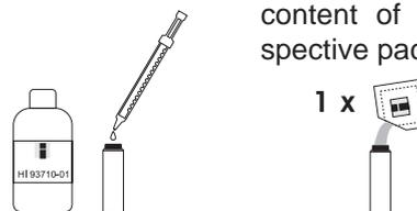
For Cyanuric Acid only, add the content of one packet of HI 93722 reagent to a beaker filled up to the 25mL mark with unreacted sample up to the 25 mL mark. Stir gently to mix and then fill the cuvet up to 1.5 cm (3/4") below the rim with 10 mL of the reacted sample.
