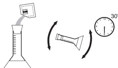
Fill a cuvet with 10 mL of the reacted sample up to 1.5 cm ( $\frac{3}{4}$ " ) below the rim and replace the cap. This is the sample.
