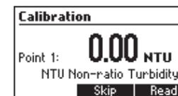
This point is used for FNU and NTU modes to check the quality of the water used for dilution and to confirm that the optical system is not dirty. In this case, if the value of the first point is over 0.15 FNU (NTU), a warning "Cal Point1 high !" is displayed when the calibration is saved and a warning "Out of calibration range" is displayed when measurements under 10.0 FNU (NTU) are performed.
