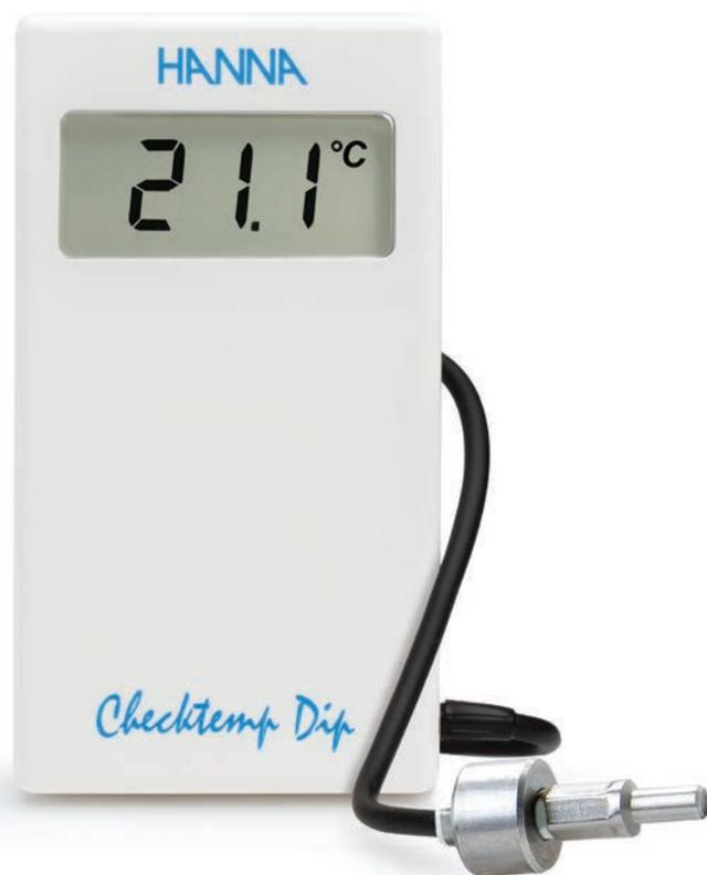
Checktemp Dip is a high-accuracy thermometer with a 3 m (9.9') flexible, silicone cable connecting the meter and the AISI 316 stainless steel weighted probe. This probe is in compliance with food regulations, making it an ideal instrument for measuring temperature in food applications such as wine casks and milk tanks. The probe incorporates an NTC thermistor sensor to measure the temperature. Thermistors make it possible to obtain extremely high accuracy in a very short period of time.
