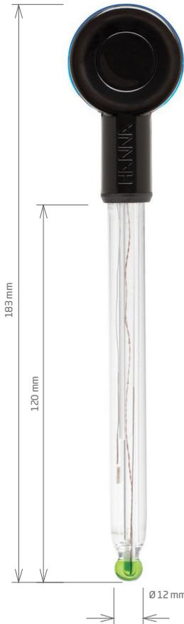
Spherical tip gives maximum surface area for fast and accurate readings
