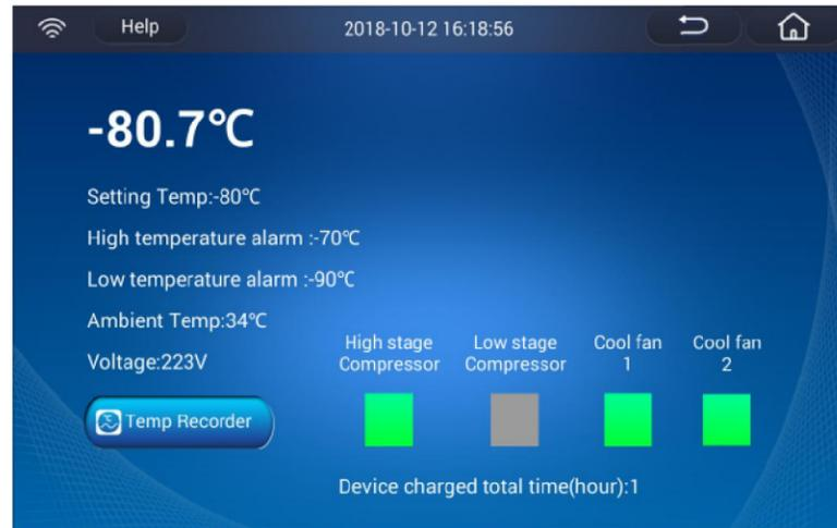
For the operation state of compressor / fan, “Green” indicates that it is running; “Grey” indicates that it is not running.
