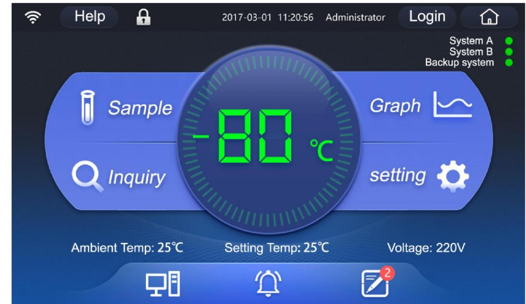
In the home page, it can display the real-time internal temperature, ambient temperature, set temperature, input voltage, backup system state (optional), network state, electromagnetic lock state (optional), user login status, freezer health status, temperature curve, and message/ note book, etc..
