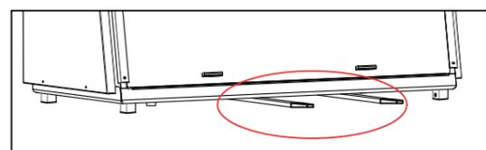
Note: For security, please use the forklift to lift the Biological safety cabinet from the rear onto the installed base shelf. Make sure the forklift arms reach the front of the cabinet before lifting, and avoid lifting the front of the work platform.
