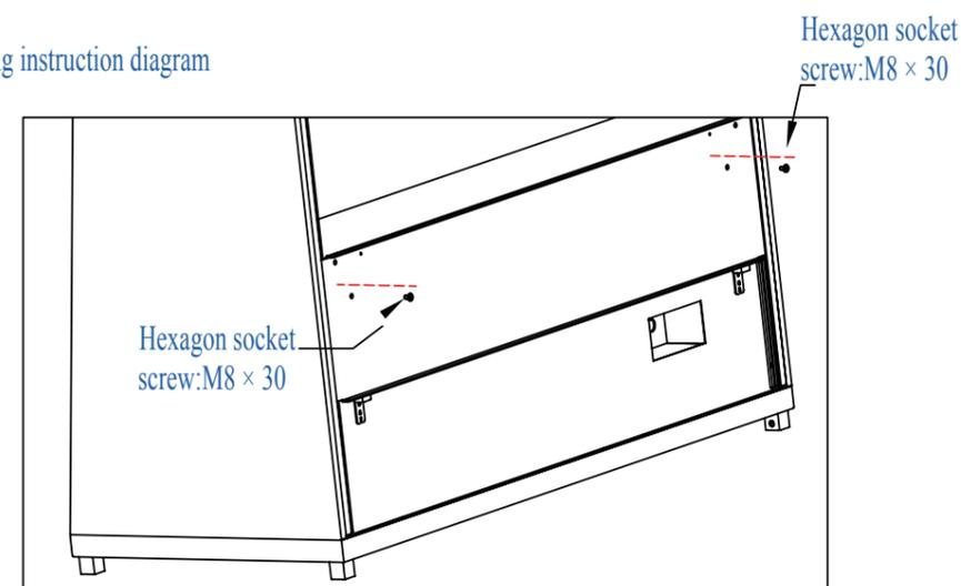
4. Before moving the cabinet body, make sure the four adjustable legs of the underframe are all on the ground to keep the underframe stable during installation, for any movement may cause safety issues. When moving the cabinet body, never put your hand at the joint between the underframe and cabinet body, so as to protect your hand from squeezing.
