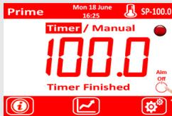
At the end of the countdown, the timer will turn the oven off. Depending on preference, you may choose to turn on a siren/beacon at this stage (selected in [Output Relay Section - Page 9](#))
