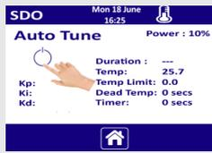
In PID mode, you can manually enter the P, I, and D value to optimise the control.
