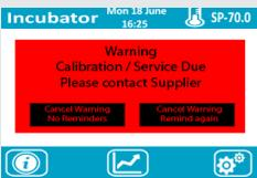
If you requested a calibration certificate with your chamber, the controller shall give you notification when the calibration /service is about to expire one month before. If you require a new calibration or service visit, please contact the supplier.
