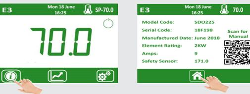
To view chamber information such as serial codes, power ratings, 2nd safety temperature value, press the
