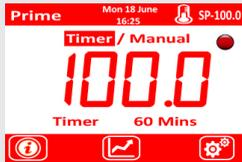
Within 2 deg of setpoint, the chamber will start the count down timer and the remain time is displayed on screen.
