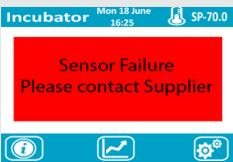
Sensor failure... If the probes fail, the chamber shall automatically turn the heating elements off. Please contact your supplier for replacement probes.
