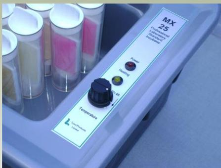
Temperature & status indicators are safe from knocks under the lid, a 37°C Quickset point helps easy initial set up
