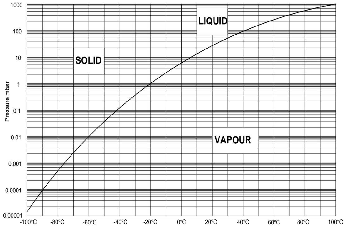
**Fig. 3.1b Vapour pressure of ice**
