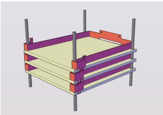
3. Push the fronts of the spacer out sideways until they come clear of the studs
