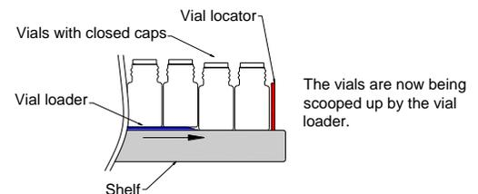
There are 6 usable shelves and each shelf holds 3 vial trays. The vial locators can hold various diameters of vials. Shelf spacers can be removed and replaced with the correct sized spacer to suit any vial height. Each of the shelves can be placed at differing heights in any combinations to suit.
