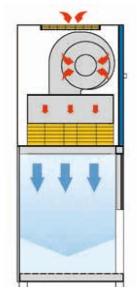
The ambient air is drawn in through the pre-filter fitted in the upper side of the cabinet and it then filtered through the HEPA filter into the work-area in laminar air flow conditions. The same volume of air is exhausted outside from the frontal aperture and under the work surface.
