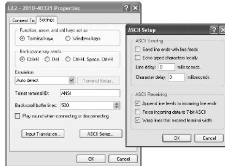
5. Enter **File | Properties | Setting | ASCII Setup** and tick **Append line feeds to incoming ends**
