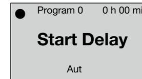
Turn the rotary switch
