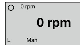
The device is in „manual“ operating mode. The speed display shows the actual and set values (=0). The single circular ring indicates that no set value has been selected.
