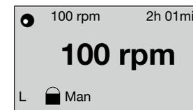
During the shaking process the above mentioned key functions can be locked by pressing the
