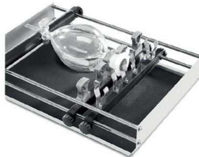
The cramp strips and spring strips are necessary for fastening separating funnels. The necks of the separating funnels are fastened in the grey plastic clamps, the spring strip secures the stoppers. The stems of the separating funnels are placed on a clamping strip h. For a modification of the standard rack system or in addition to the clamping strips h.
