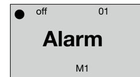
The submenu 01 alarm appears on the display. In this submenu the multiple alarm can be activated or deactivated. At the upper left the active setting is indicated. At the upper right the number of the submenu is displayed.
