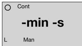
Press the page key (P) to change to the time display. „Cont“ is displayed for the set value, i.e. the shaker is running continuously. The main display shows -min -s.
