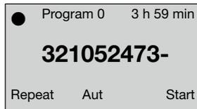
When the device is switched on, the operating mode which was active before it was switched off is activated again. In this example program 0 was active.
