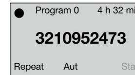
„Start“ and the remaining time are flashing alternately until the start. The program can also be started immediately by pressing the
