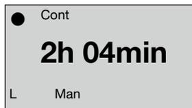
Turn the rotary switch (OK) to select the running time. If the running time surpasses 59min 59s, the time display switches from „mm ss“ to mode „hh mm“. The max. possible operation with timer is 99h 59min.
