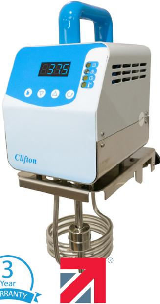
Clifton Range NE4-SB features a digital PID temperature controller which provides even water circulation and temperature stability.
