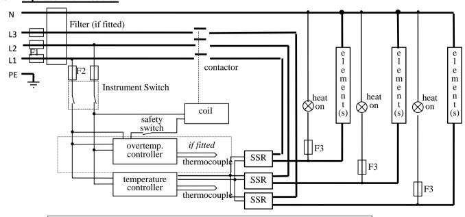
note on (2- and) 3-phase: depending on filter(s) fitted, there may be (2 or) 3 separate neutral wires from the elements to the neutral supply.
