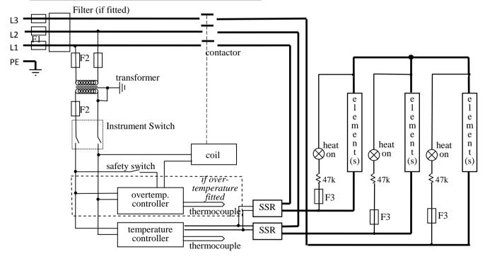
Note: in this configuration the fuses F2 on the supply side of the transformer may be GEC Safeclip, not  $32 \times 6$ mm glass as stated in section 8.1.
