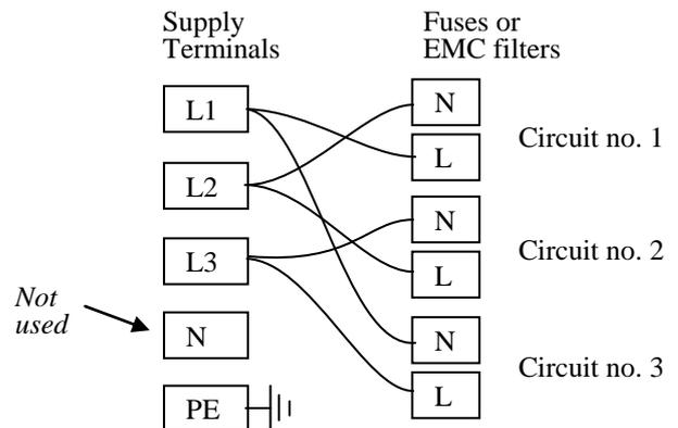
A model made to this diagram can be converted by the customer between the following supply voltages:
