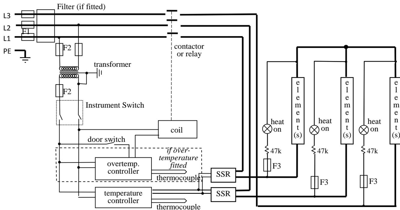
In this configuration the fuses F2 on the supply side of the transformer may be GEC Safeclip, not 32 x 6mm glass as stated in section 8.0.
