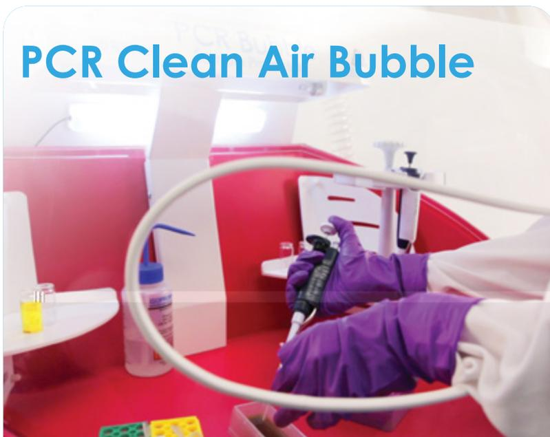
The PCR Clean Air Bubble provides a comfortable to use, easy to clean, HEPA filtered clean air environment for the preparation of PCR reagents. The integrated UV-C Germicidal Lamp provides effective bio-decontamination.
