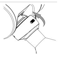
▶ Remove the evaporating flask from the vapor duct.
