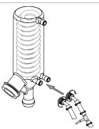
▶ Plug the sensor cable into the Rotavapor® connection **CW/T**.
