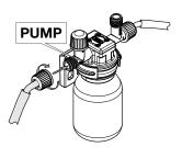
► Attach the hose to the vacuum pump connection IN
