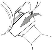
▶ Open the Combi-Clip to release the flask.
