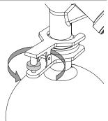
▶ Remove the ball joint clamp.
