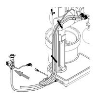
▶ Plug the cable from the cooling water valve into the available connection on the cooling water temperature sensor or to the Rotavapor® connection **CW/T**.
