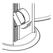
▶ Move the height adjustment stopper right below the rotary drive arm.
