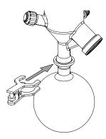
▶ Turn the wheel to secure the ball joint clamp.
