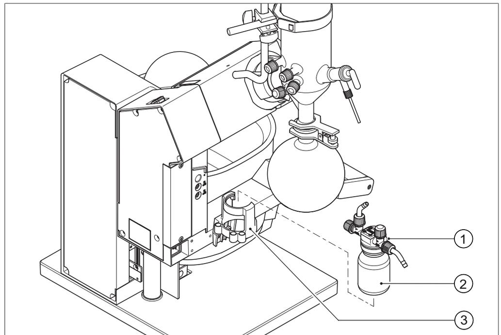
Fig. 12: Mounting the Woulff bottle on the Rotavapor
