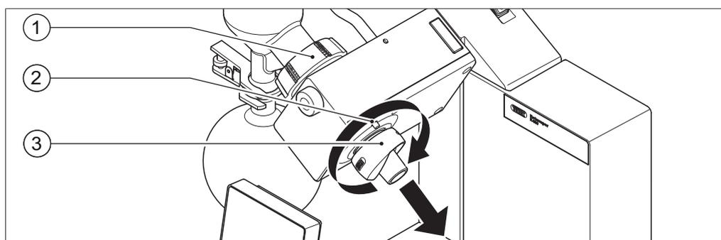
Fig. 45: Vapor duct on Rotavapor R-300
