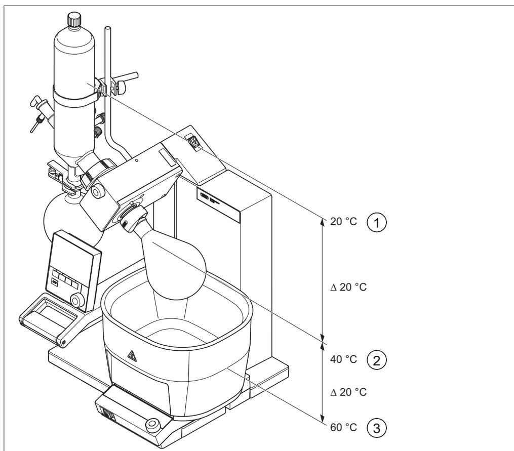
Fig. 40: Distillation conditions
