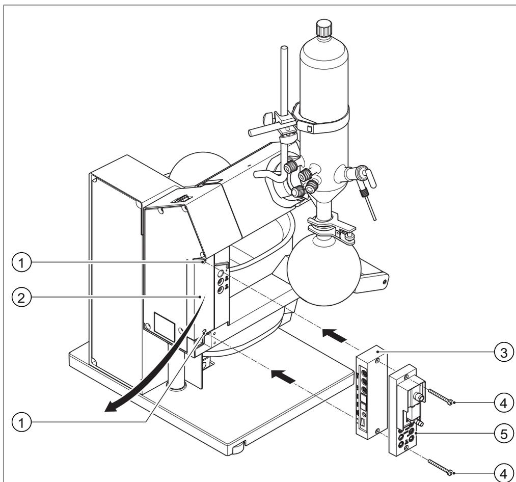
Fig. 11: Mounting LegacyBox and VacuBox on the Rotavapor
