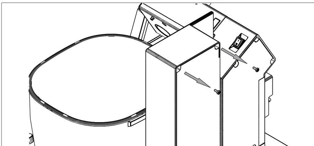
Fig. 19: Removing the screws on the rear panel
