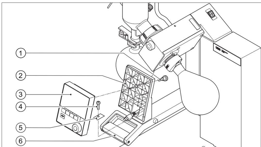
Fig. 9: Fitting the holder and interface unit on the handle
