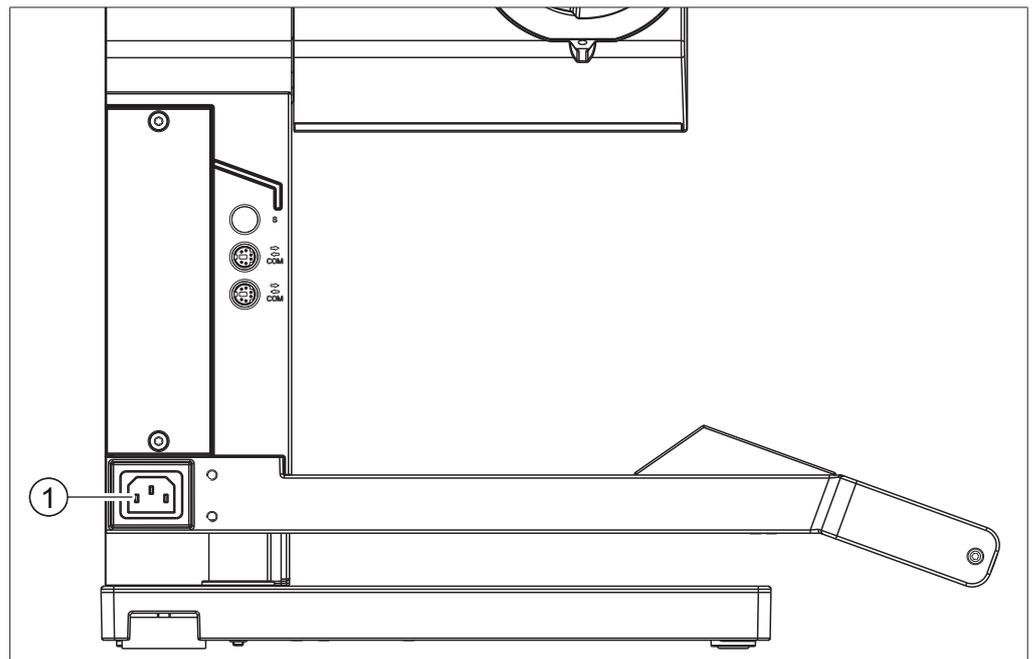
Fig. 22: Power supply connection on Rotavapor R-300
