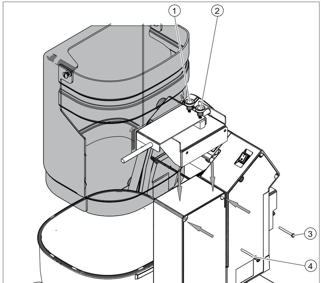
Fig. 20: Fitting the splash guard on the Rotavapor
