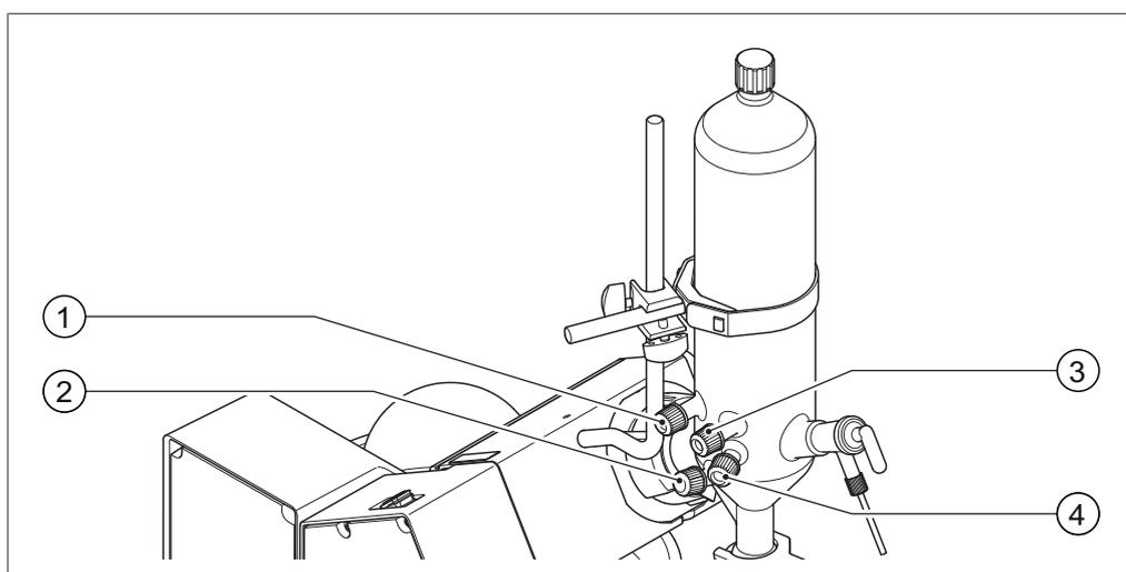
Fig. 15: Vacuum and coolant tubing connections on the cooling condenser of the R-300
