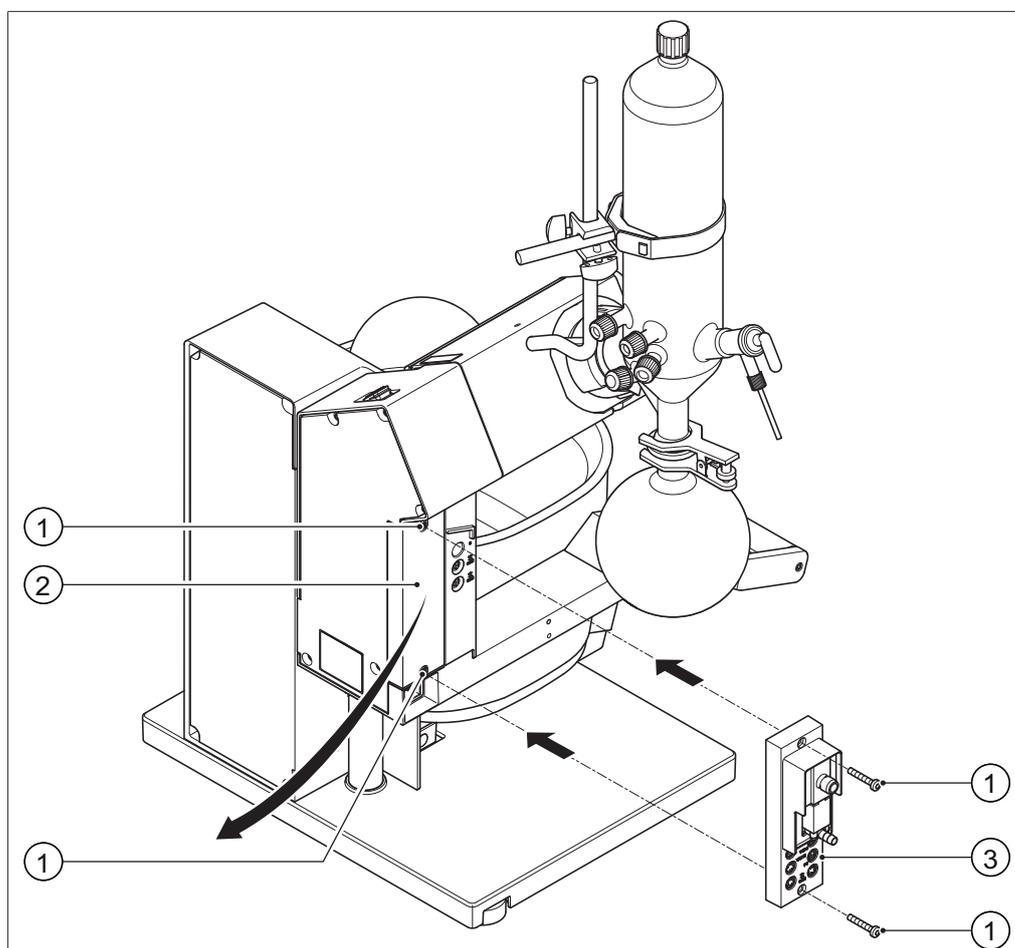
Fig. 10: Mounting the VacuBox on the Rotavapor
