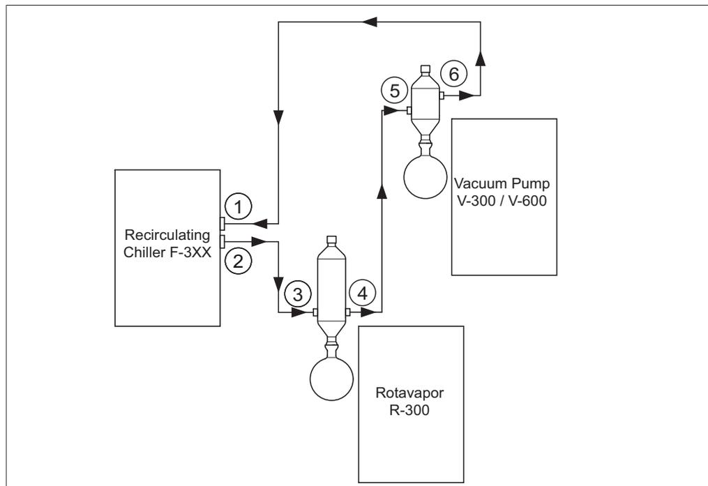
Fig. 27: Coolant tubing connections in a BUCHI distillation system (example)
