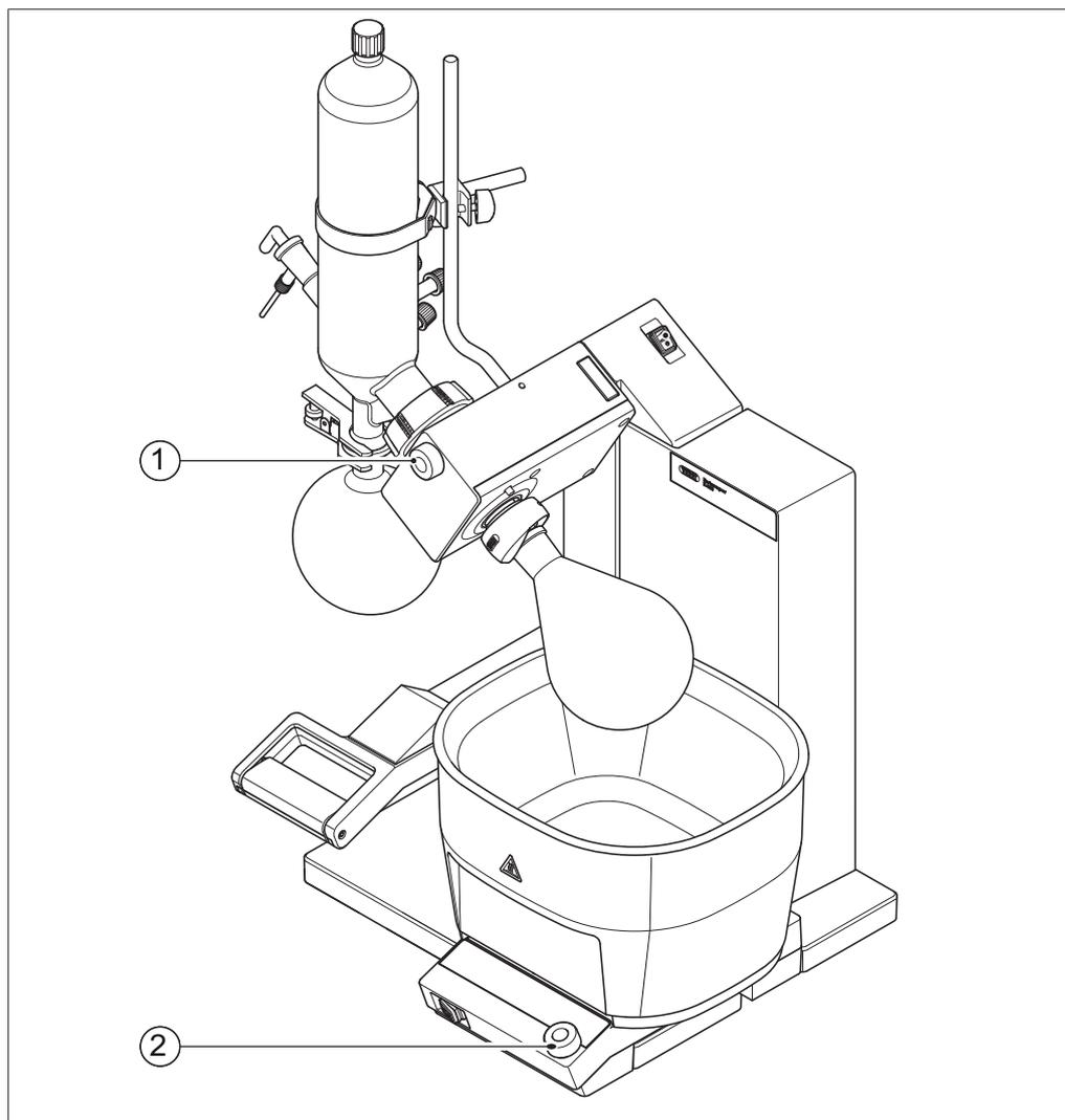
Fig. 38: Components for manual control of Rotavapor R-300
