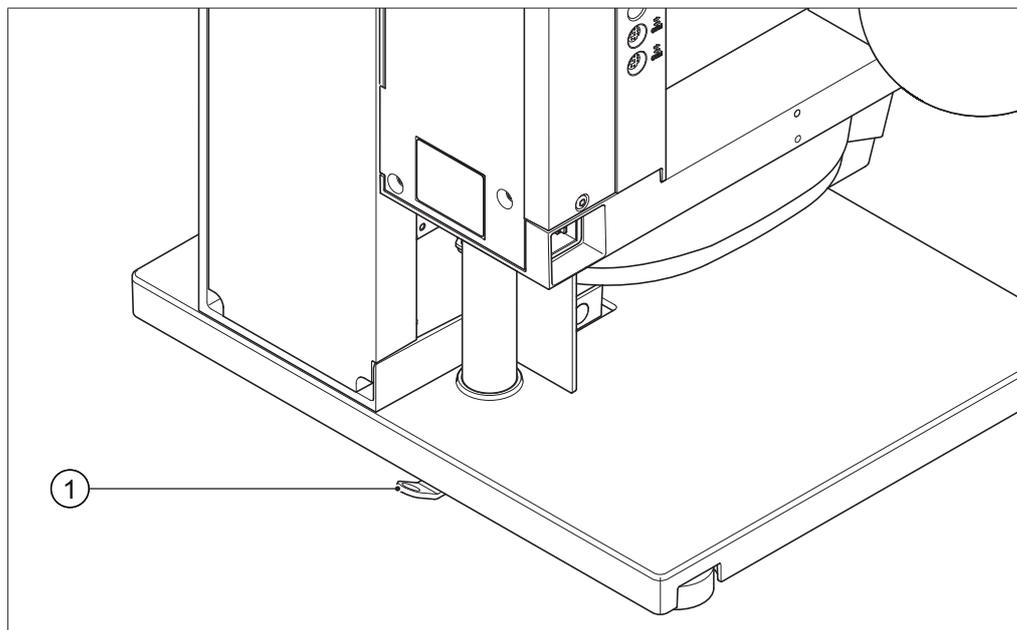
Fig. 6: Earthquake fixing
