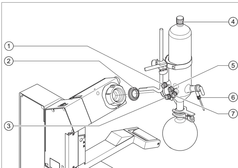
Fig. 47: Seals on Rotavapor and cooling condenser
