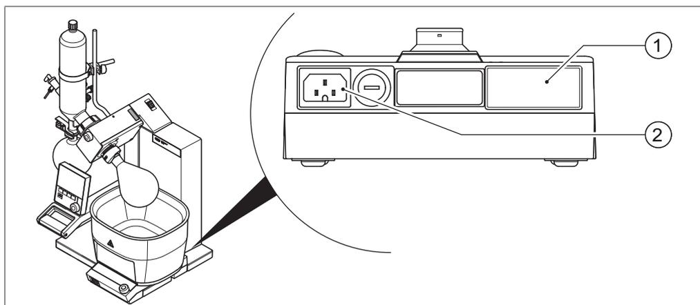
Fig. 23: Power supply connection on heating bath base
