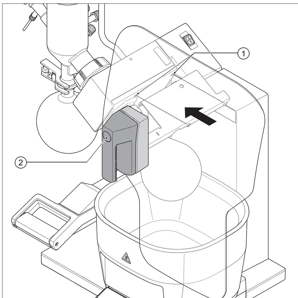
Fig. 18: Fitting the protection shield on the Rotavapor
