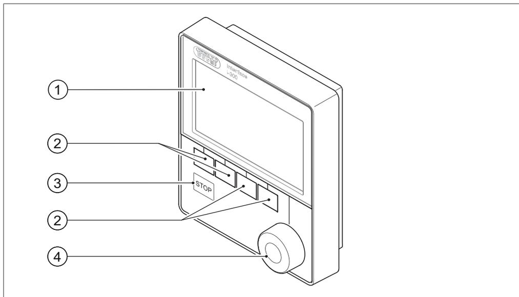
Fig. 39: Front view of Interface I-300 showing controls
