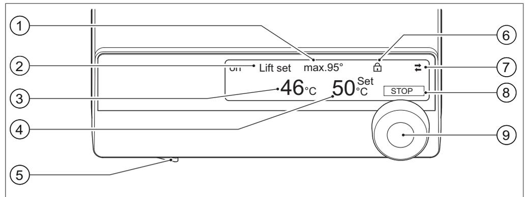
Fig. 3: User interface of Heating Bath B-300 Base
