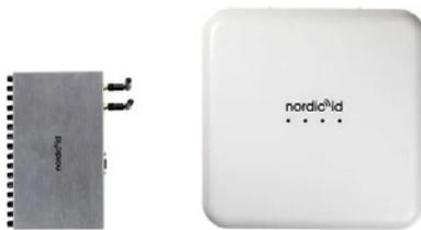
Before a shipment of blood tubes is sent to a partner lab for analysis, it is placed in a custom 'shipment box', equipped with fixed AR 62 RFID scanners. Scanned data are displayed on the shipment box and sent to the customer's ERP system to indicate which blood tubes are about to be shipped.
