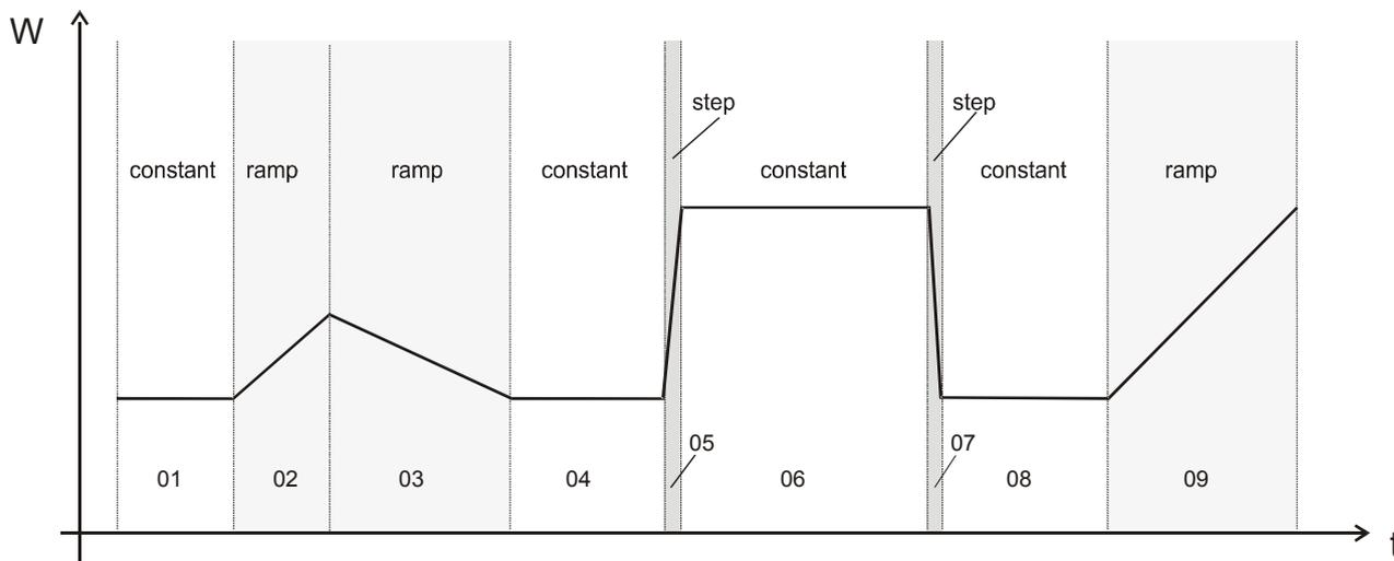
Figure 7: Possible temperature transitions
