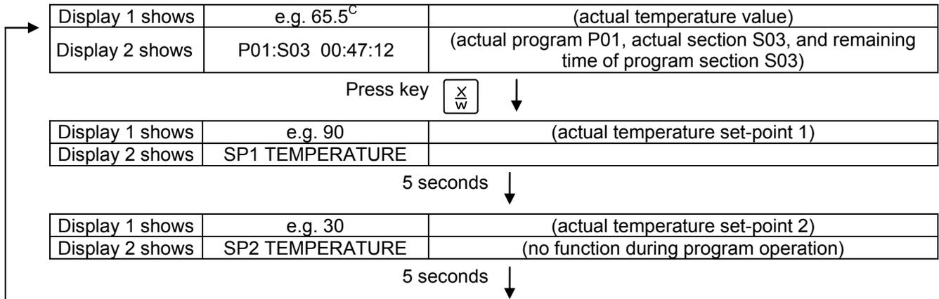
After program runoff (and, if appropriate, of the program repeats) the controller returns to fixed value operation showing Normal Display and adjusting to the temperature value that has been previously entered in the fixed value entry mode.
