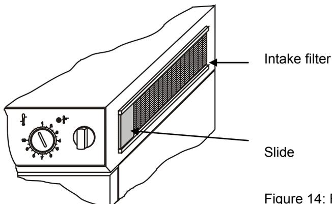
Figure 14: Fresh air intake filter
