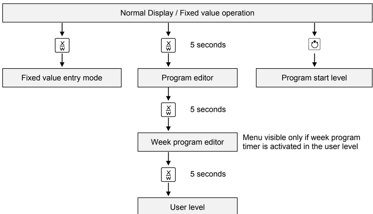
If no button is touched within more than 120 sec. the controller returns from the current level to Normal Display.
