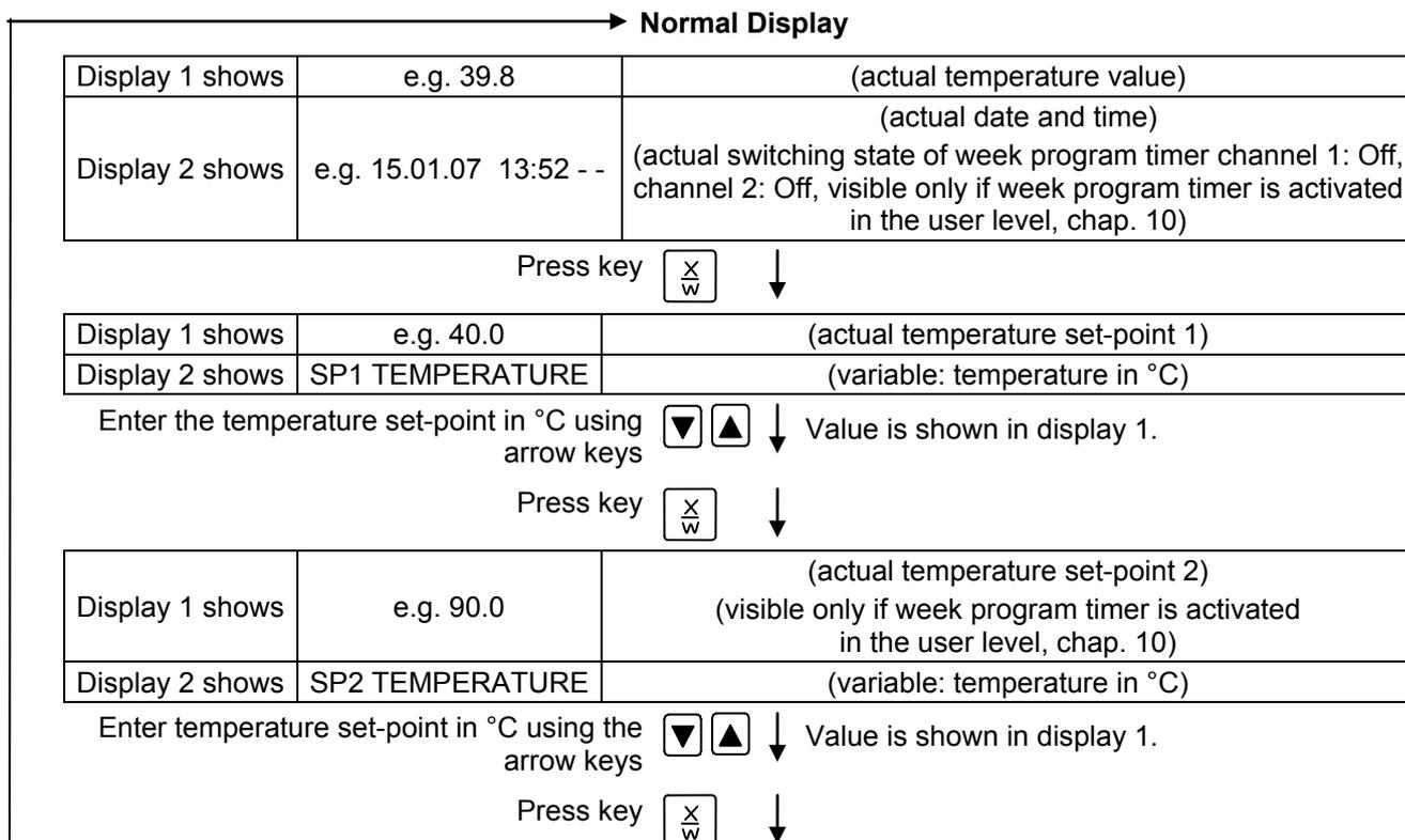
If no button is pressed within more than 120 sec, or if the EXIT button is pressed, the controller changes to Normal Display.
