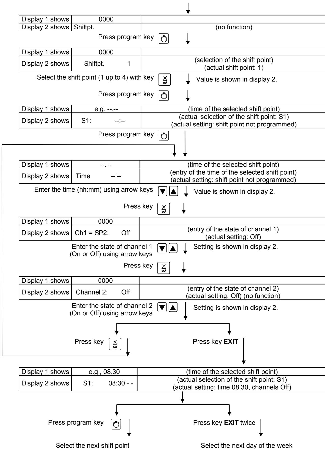
To exit the menu, press several times key **EXIT** or wait for 120 seconds. Controller returns to normal display.
