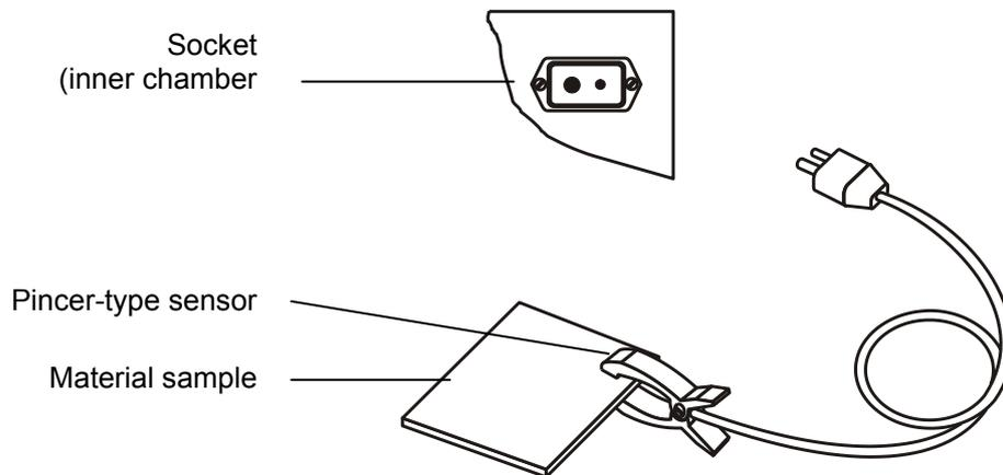
Figure 12: Sensor probes for optional temperature display
