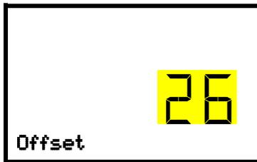
Setting the safety controller value with “Offset” safety controller mode
