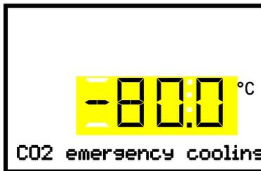
Setting the CO<sub>2</sub> emergency cooling temperature setpoint
