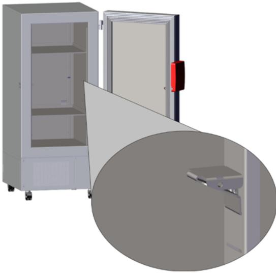
Figure 17: Inserting the shelf holders
