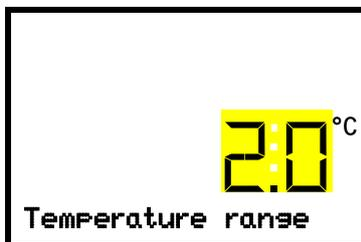
Setting the temperature tolerance range
