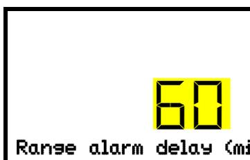
Setting the tolerance range alarm delay.
