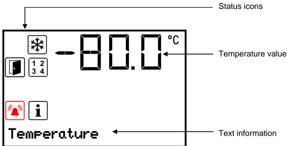
Figure 21: Normal display of the RD4 controller (sample values)
