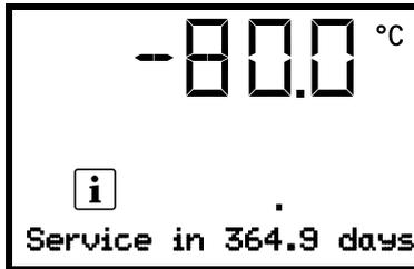
The remaining time in days until maintenance is due is shown in the text field of the controller display.
