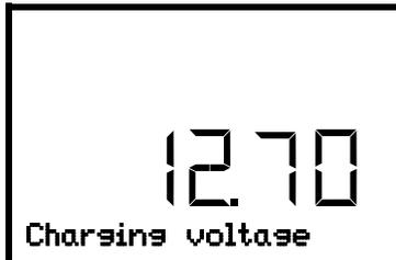
Display of the battery's current charging voltage.
