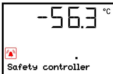
Alarm indication (example: safety controller alarm)
