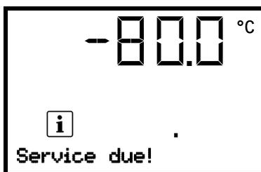
The message "Service due!" is shown in the text field of the controller display.
