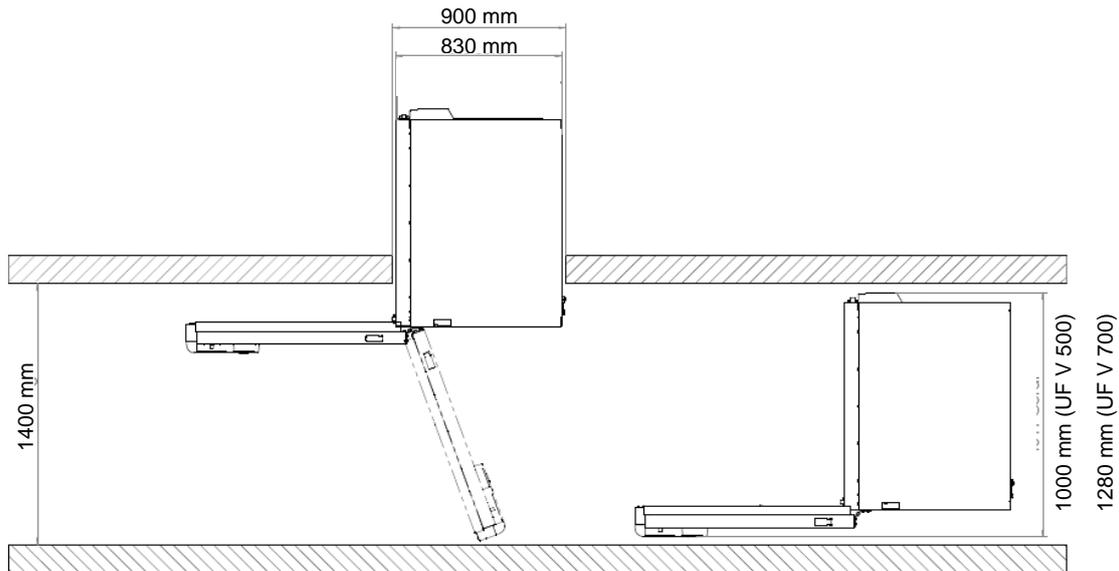
Figure 14: UF V with open chamber door
