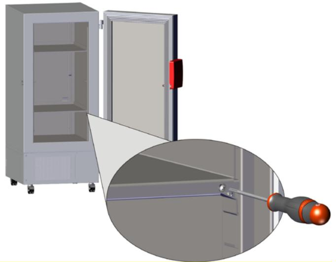
Figure 18: Screwing the shelves to the shelf holders
