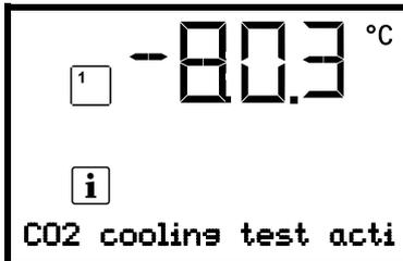
Information message (example: CO<sub>2</sub> emergency cooling test run is active)
