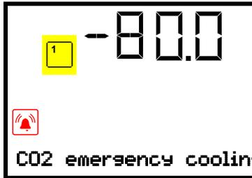
Normal display with running emergency cooling, showing the alarm message "CO2 emergency cooling"
