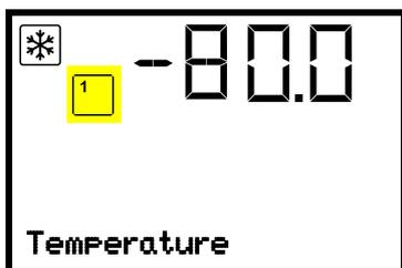
Normal display with activated emergency cooling
