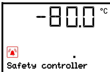
Normal display showing safety controller alarm (sample value)
