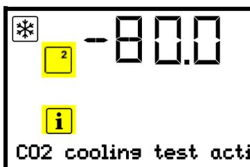
Normal display during test run of the CO<sub>2</sub> emergency cooling, showing the information message "CO2 cooling test active"
