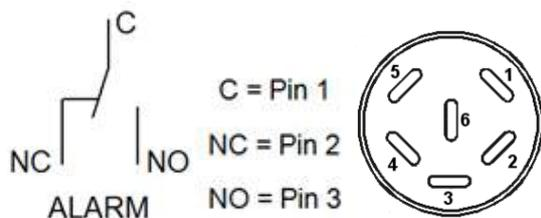
Figure 22: Zero-voltage contacts circuit diagram and pin allocation of DIN socket (8)
