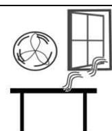
Do not place near open windows, air-conditioning vents or fans that may cause a draft and unstable readings.
