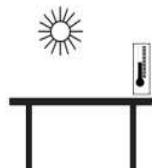
Avoid extremes of temperature. Do not place in direct sunlight or near air conditioning vents.
