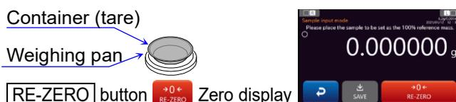
Step 2. Place the specified number of sample pieces on the container/weighing pan.
