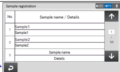
Step 6. Register the first sample in the recipe. Select the desired sample using the **Selection** button, and then enter values in the [Target value] and [Tolerance] fields. In the example, the sample name is Sample1, the target value is 1.000000 g, and the tolerance is 10.000%. After inputting, press the right arrow button **→** at the bottom right of the screen to display the registration screen for the second sample.
