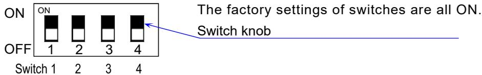
The factory settings of switches are all ON (upper side). It means static elimination method is in 'timer mode,' 'discharging time' is for 3 seconds, and 'built-in IR sensor' and 'buzzer' are available.
