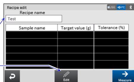
Step 4. Select the sample to be registered using the **Selection** button in the [Sample name] field.
