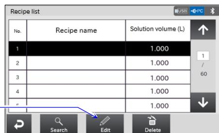
Step 3. Enter the recipe name. In the example, the recipe name is set to "PBS (-)", the buffer volume is set to 1.000 L, and the target value unit is set to mmol/L. After setting, press the **Edit** button to display the [Sample edit] screen in step 4.
