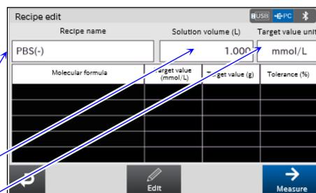
Step 4. Select the sample to be registered using the **Selection** button in the [Molecular formula] field. To select a sample other than the one registered at the time of shipment from the factory, the sample needs to be added to the **Selection** button. In this case, press the **Add sample** button to go to the [Sample registration] screen in step 5. In this example, potassium chloride is newly registered. Press the **Add sample** button to go to step 5.
