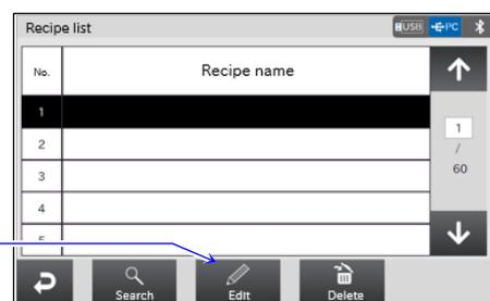
Step 3. Enter the recipe name. In the example, the recipe name is set to "Test". After inputting, press the **Edit** button to display the [Sample edit] screen in step 4.
