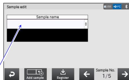
Step 5. Enter the [Sample name] and [Details] to be registered. The figure on the right shows an input example on the [Sample registration] screen. After inputting, press the **Back** button to display the [Sample edit] screen.
