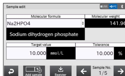
Step 7. Enter the contents of the remaining samples in the same way. Then, press the **Register** button to register the recipe and to display the [Recipe edit] screen.
