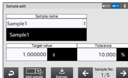
Step 7. Register the second sample in the recipe. Enter values in the [Target value] and [Tolerance] fields. Then, press the **Register** button to register the recipe and display the [Recipe edit] screen.
