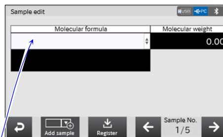
Step 5. Enter the [Molecular formula] and [Sample name] to be registered. The figure on the right shows an input example on the [Sample registration] screen. After inputting, press the **Back** button to display the [Sample edit] screen.
