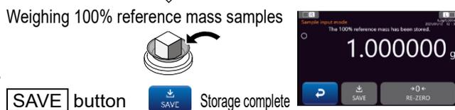
Step 3. Press the [SAVE] button
