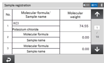
Step 6. Register the first sample in the recipe. Select the desired sample using the **Selection** button, and then enter values in the [Target value] and [Tolerance] fields. In the example, the sample name is Na<sub>2</sub>HPO<sub>4</sub>, the target value is 10.000 mmol/L, and the tolerance is 10.000 %. After inputting, press the right arrow button **→** at the bottom right of the screen to display the registration screen for the second sample.
