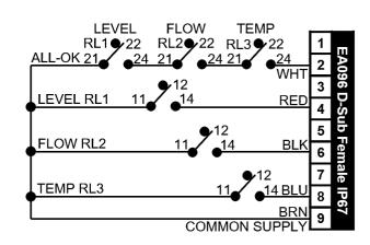
Dependent on your product type, signals will either be accessible via a standard two-row 9-pin D subminiature connector (see below left) OR direct connection to terminal blocks (see below right). Where a D connector is provided, the female gender (ATC PN EA096) is supplied in all cases. If male pins are required, we recommend using a male-to-male gender-changer connector (ATC PN EA853). Pin numbers are clearly marked on the molding. The connector is rated to IP67.
