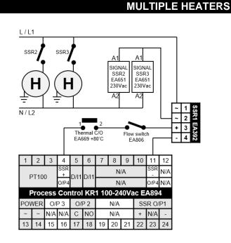
contact side capable of supporting the current pulled by two heaters in parallel.
