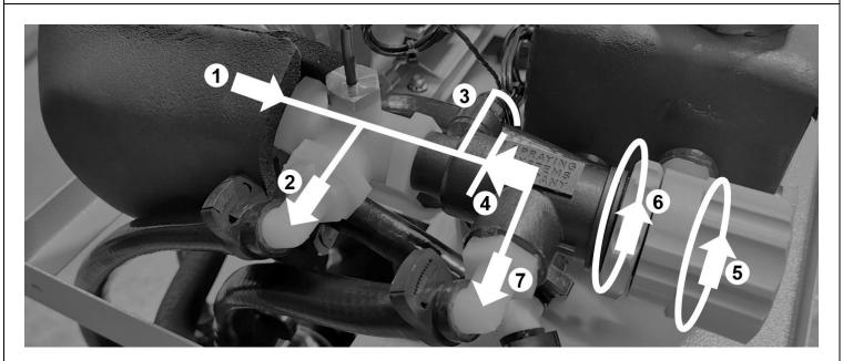
It is important to understand the basic principle that all else being equal, higher flow results in a higher demand for pressure. The motor generates the power required to turn the pump head and create that pressure. The more restrictive a water circuit is, the higher the pressure required to maintain flowrate. Positive displacement pumps are designed to generate high pressure and are mechanically tight - their RPM dictates flowrate. See image;
