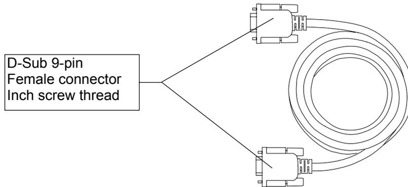
Use the waterproof RS-232C cable (AX-KO2737-500) that is sold separately as an option, when the RS-232C serial interface is used with IP-65. (Refer to page 67)
