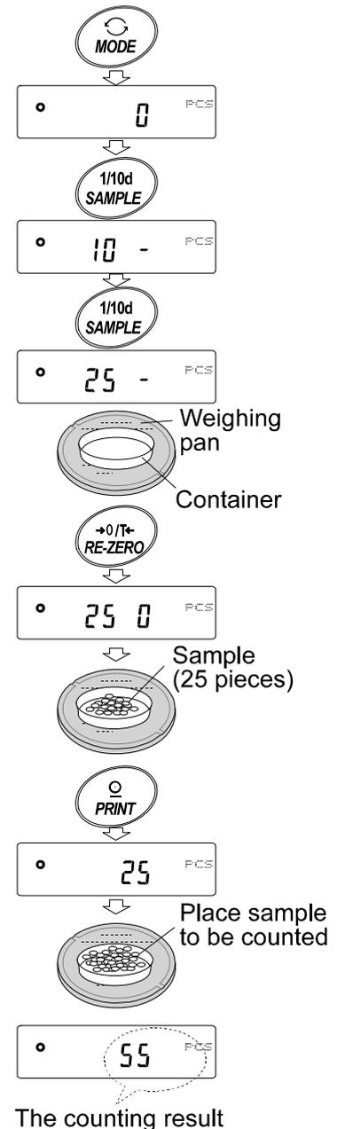
If the balance judges that the mass of the samples is too light to acquire accurate weighing, it displays an error requiring the addition of more samples to the specified number. In the example above, **50-PCS** appears, requiring 25 more samples. Add 25 samples and press the **PRINT** key. When the unit mass is stored correctly, the balance proceeds to the counting mode.
