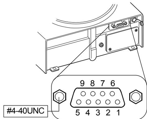
Signal names of the balance side are the same as the DTE side with TXD and RXD reversed.
