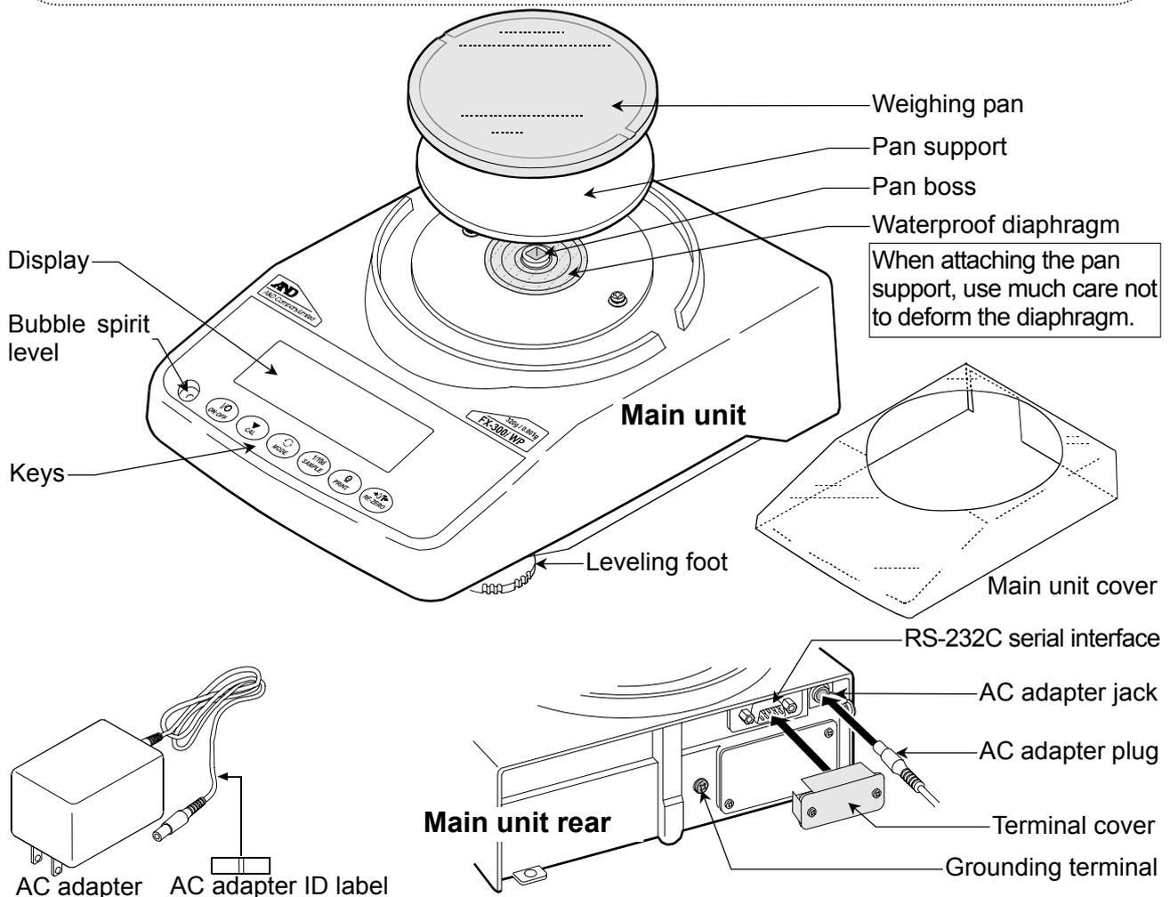
When attaching the pan support, use much care not to deform the diaphragm.
