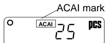
8. After setting the unit weight at step 6, add a few more samples on the pan. Then, the ACAI mark will turn on. (Add more than three pieces. The mark will not turn on for the number of samples beyond the ACAI range.)
