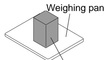
5. Press the **PRINT** key to store the reference weight. Remove the sample.
