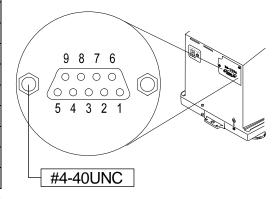
Signal names of the balance side are the same as the DTE side with TXD and RXD reversed.
