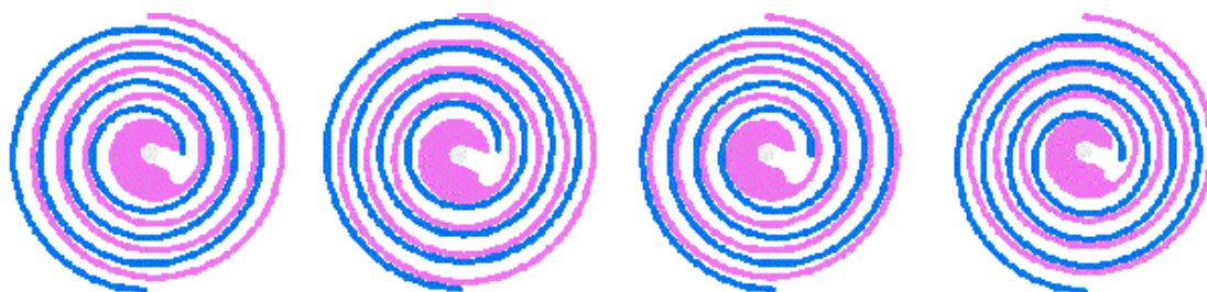
Fig. 2 Working principle of the Scroll pump
