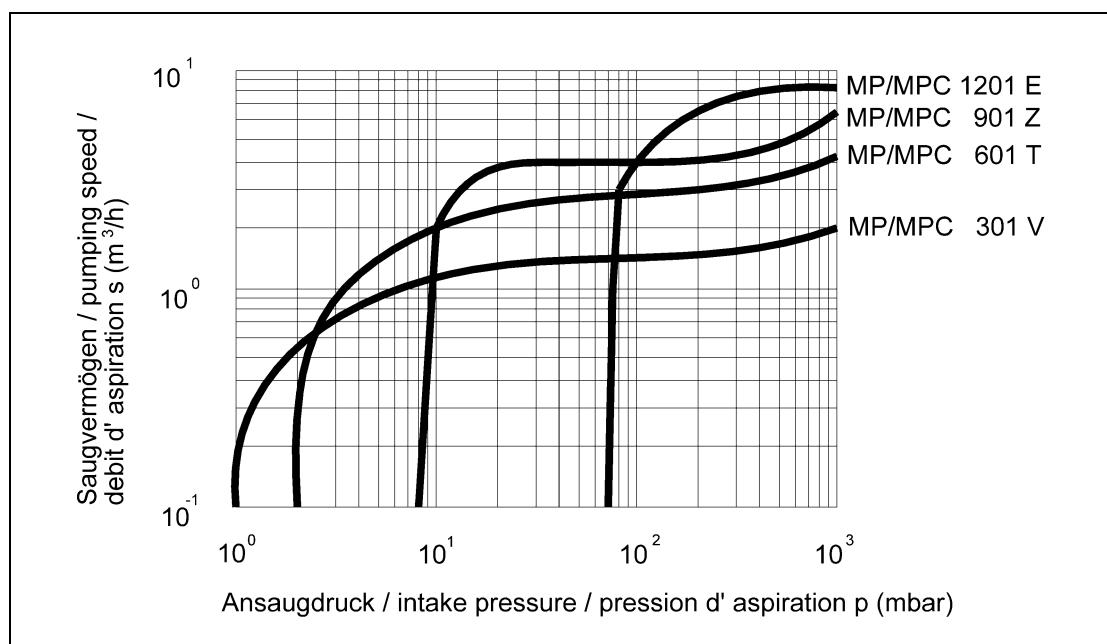
Fig. 4 Intake Pressure / Pumping Speed - Diagram
