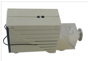
In-Line Safety valve Type VA 25 ME The automatic in-line safety valve is connected with the intake of the scroll pump. It closes the intake flange when the pump is voluntarily or accidentally shut down, thus maintaining the vacuum in the connected system. The in-line safety valve is opened electromagnetically.
