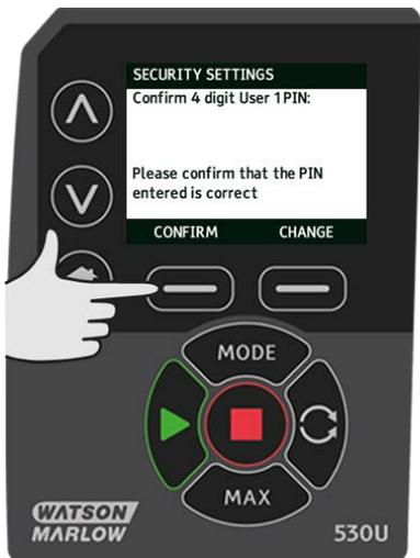
To define the allowed functionality, use the ^/∨ keys to select the functionality and press **ENABLE**. User 1 PIN will allow access to only the enabled functionality, to disable functionality, highlight the enabled functionality and press **DISABLE**. When all the required functionality has been enabled, press **FINISH**.
