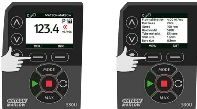
This will display the main menu as shown below. Use the  $\wedge$  /  $\vee$  keys to move the selection bar between the available options.
