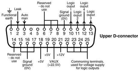
Recommended control cable: 7/0.2mm 24AWG screened. Cable screen should be earthed with a 360 deg connection to a conductive back-shell. This will be connected to pump mains EARTH via the D connector body. Mains Earth is also available on pin 1 Upper D and pin 13 Lower D.
