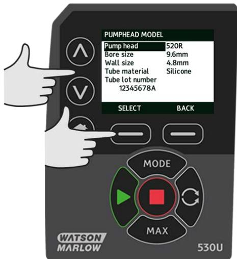
Use the  $\wedge$  /  $\vee$  keys to move the selection bar over the tube size to be used and press **SELECT**.
