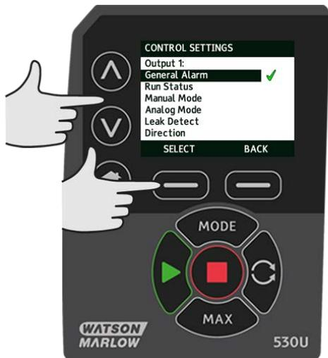
Use the ^ /v keys and press **SELECT** to choose the logic state of the chosen output. Press **SELECT** to program the output or **BACK** to cancel.
