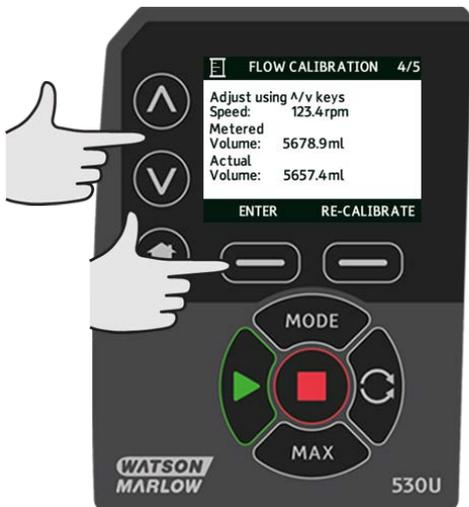
To accept the new calibration press **ACCEPT** or **RE-CALIBRATE** to repeat the procedure. Press **HOME** or **MODE** to abort.
