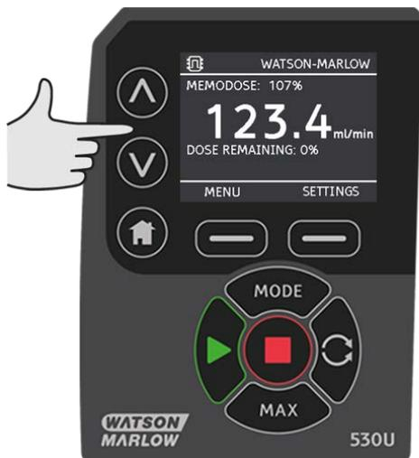
If **STOP** is pressed during dosing, the pump stops. Pressing **START** will resume, or discard, the interrupted dose depending on the settings in "MemoDose mode" on page 57.
