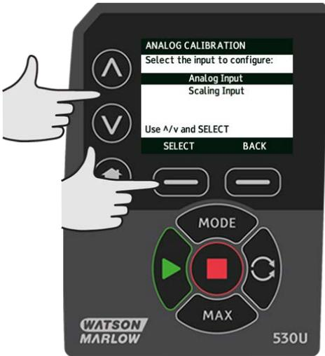
Select the input signal type using the  $\wedge$ / $\vee$  keys and press **SELECT**.
