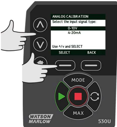
The pump gives the option to enter the high and low mA or V signals manually or via the analog input. Entering mA values is described here, however the process for entering V signals is identical.
