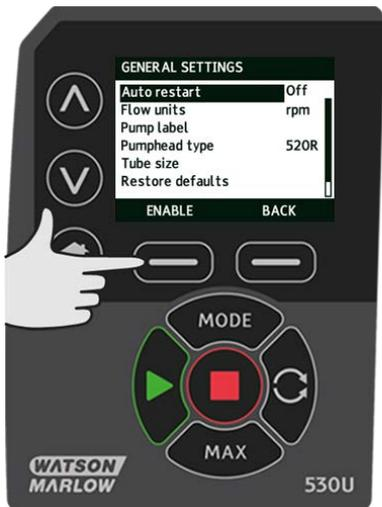
Use the  $\wedge$  /  $\vee$  keys to move the selection bar over **Pumphead** and press **SELECT**.
