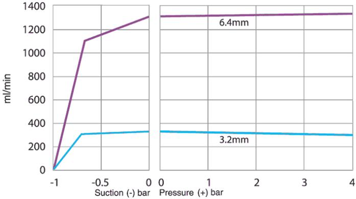
**Sta-Pure element, 2-4 bar (30-60psi), 200rpm, counter-clockwise rotation**
