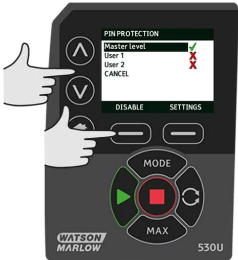
ENABLE user 1 security settings displays the PIN entry screen for User 1. To define a four digit User 1 PIN, use the ^/∨ keys to select each digit from 0-9. Once you have the required digit press the **NEXT DIGIT** key. After selecting the fourth digit press **ENTER**.
