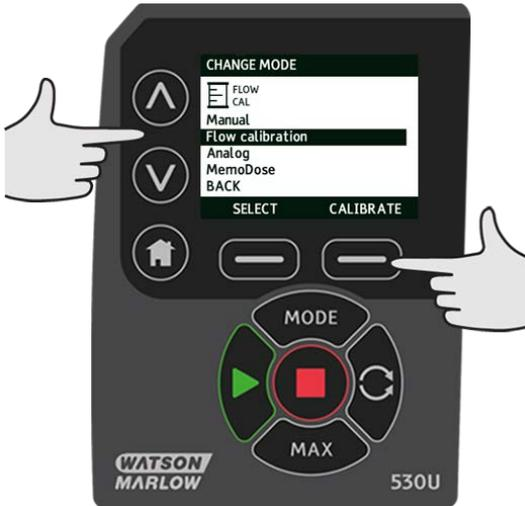
Using the  $\wedge$ / $\vee$  keys, enter the maximum flow rate limit and press **ENTER**.
