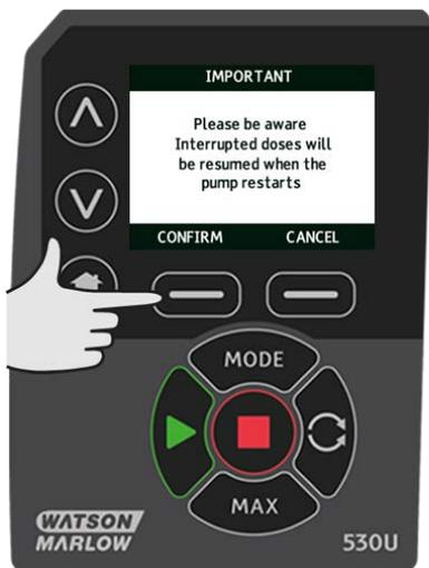
If resume interrupted doses has NOT been set the following warning screen is displayed, press **CONFIRM** to save this setting.
