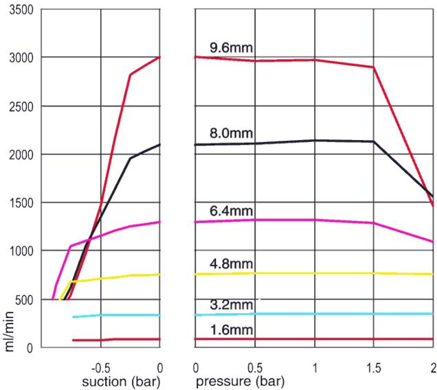
**Marpene continuous tubing, 2.4mm wall, 200rpm, counter-clockwise rotation**
