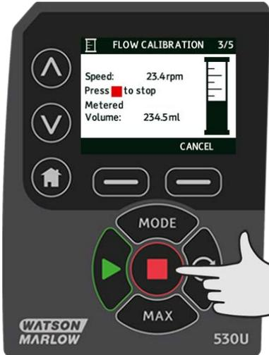
Use the  $\wedge$  /  $\vee$  keys to enter the actual volume of fluid pumped.
