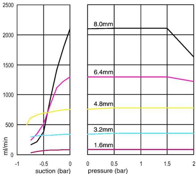
**Marprene continuous tubing, 1.6mm wall, 200rpm, counter-clockwise rotation**
