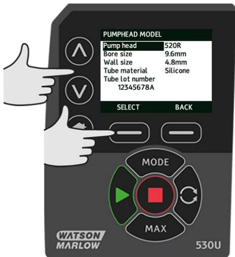
Use the  $\wedge$  /  $\vee$  keys to move the selection bar over the tube material to be used and press **SELECT**.
