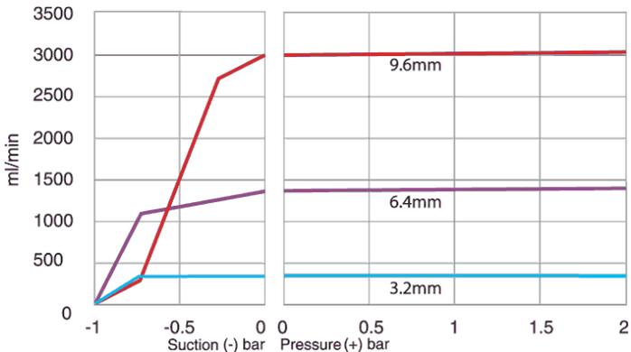
**Sta-Pure element, 0-2 bar (0-30psi), 200rpm, counter-clockwise rotation**
