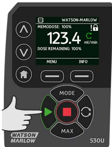
If the delivered dose differs from the volume required, the percentage may be adjusted within the limits 1% to 999% of the master dose. Use the  $\wedge$ / $\vee$  keys to alter the percentage. The new dose size is displayed as a percentage on the home screen.
