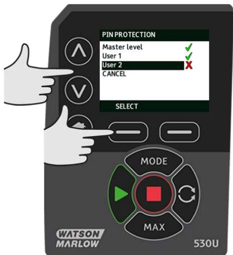
ENABLE user 2 security settings displays the PIN entry screen for User 2. To define a four digit User 2 PIN, use the  $\wedge$ / $\vee$  keys to select each digit from 0-9. Once you have the required digit press the **NEXT DIGIT** key. After selecting the fourth digit press **ENTER**.
