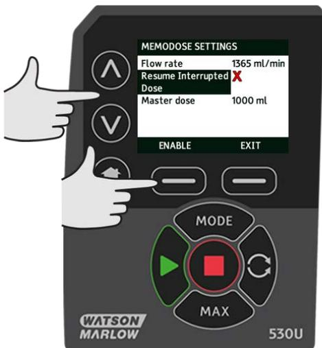
If resume interrupted doses has been set the following warning screen is displayed, press **CONFIRM** to save this setting.
