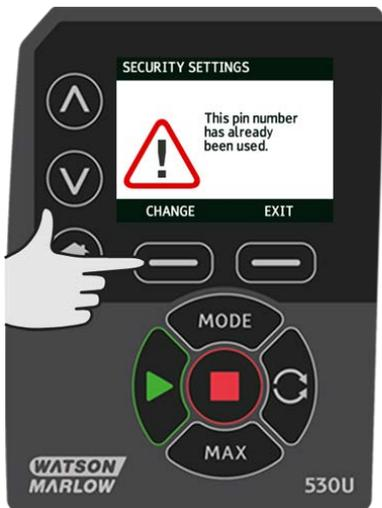
If the PIN entered does not allow access to the functionality the following screen will be displayed.
