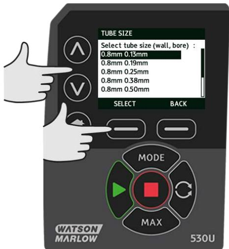
If a LoadSure element has been selected then the tube size is displayed as pressure and bore.
