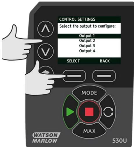
Use the ^ /v keys and press **SELECT** to choose which pump status you require for the chosen output. The tick symbol indicates the current setting.
