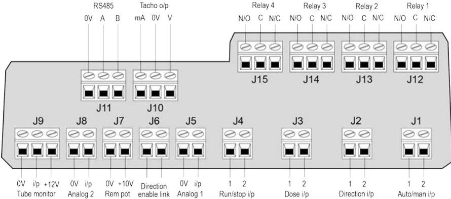
Recommended control cable: metric = 0.14sq mm - 2.5sq mm solid and 0.14sq mm - 1.5sq mm stranded. USA = 26AWG - 14AWG solid and 26AWG - 16AWG stranded. Cable: circular. Max/min outside diameter to ensure a seal when passed through the standard gland: 9.5mm-5mm. **The cable section must be circular to ensure a seal.**
