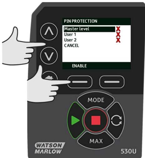
To define a four digit Master PIN, use the  $\wedge$  /  $\vee$  keys to select each digit from 0-9. Once you have the required digit press the **NEXT DIGIT** key. After selecting the fourth digit press **ENTER**.
