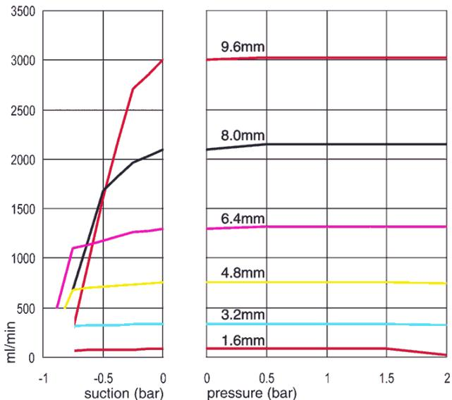
**Marpene TL element, 0-2 bar (0-30psi), 200rpm, counter-clockwise rotation**
