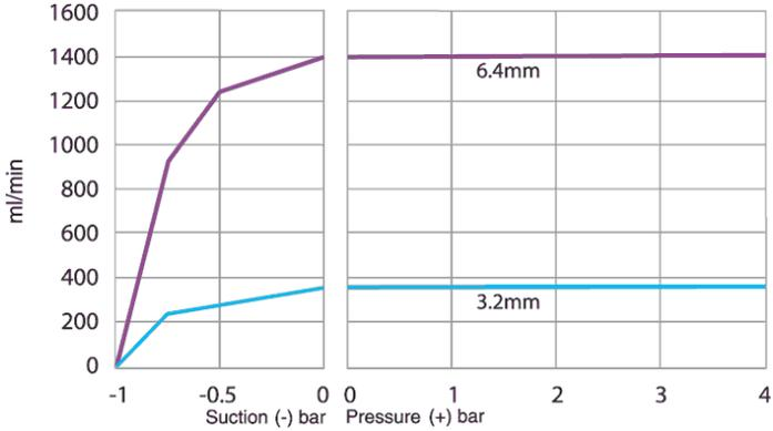
**Marprene TH element, 4-7 bar(60-100psi), 200rpm, counter-clockwise rotation**
