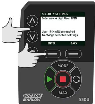
Now press **CONFIRM** to check that the number entered is the PIN you require. Press **CHANGE** to return to PIN entry.
