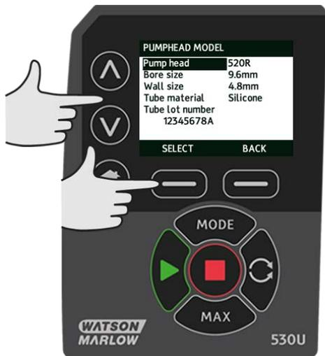
Use the  $\wedge$  /  $\vee$  keys to move the selection bar over the required pumphead type and press **SELECT**.
