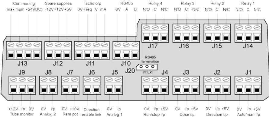
Recommended control cable: metric = 0.14sq mm - 2.5sq mm solid and 0.14sq mm - 1.5sq mm stranded. USA = 26AWG - 14AWG solid and 26AWG - 16AWG stranded. Cable: circular. Max/min outside diameter to ensure a seal when passed through the standard gland: 9.5mm-5mm. **The cable section must be circular to ensure a seal.**
