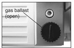
For **condensable vapors** (water vapor, solvents, etc.):
