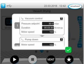
VACUU·SELECT includes predefined vacuum procedures for all common lab applications. The process steps and control parameters can easily be adjusted to suit any application.
