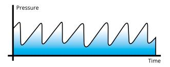
The vacuum controller switches a vacuum valve on and off, holding the vacuum level stable within a tight range or hysteresis. VACUU·SELECT automatically adjusts the hysteresis based on process demands in order to minimize pressure fluctuations and maintain process control. This is especially important for evaporative processes, where the hysteresis is automatically set based on the first vapor pressure detected.
