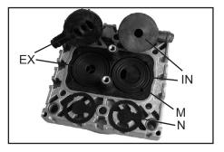
Insert O-rings (M) and valves (N). See figure for the correct position of the valves:
