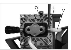
Detach the coupling of the connection tube (V) to the other side of the pump at the valve head (O).
