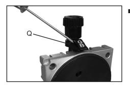
Open the hinged cover of the connection fastener (Q) with a slotted screwdriver.
