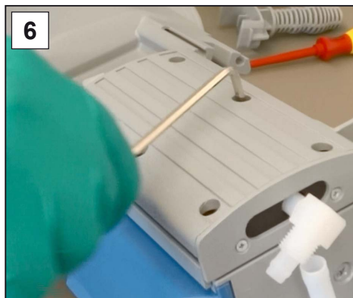
6. Place the housing cover as well and screw in the screw connections; Allen key 4, tightening torque, 6 Nm.
