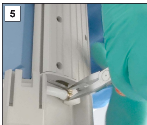
5. Close the open hose clamps using the flat nose pliers.
