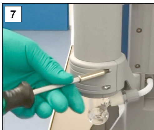
7. Secure the counterholder; Torx screwdriver TX10. For EKP or TE, screw on the retaining plate; Phillips screwdriver 2.
