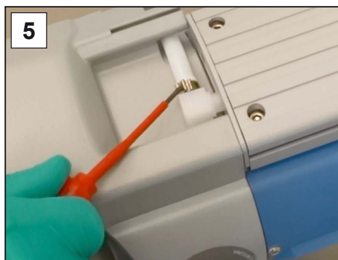
5. Open the hose clamp; flat-head screwdriver 1.
