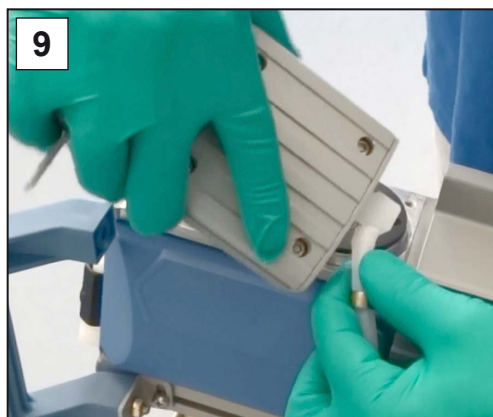
7. Lift the housing cover and remove the molded hose.
