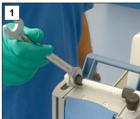
1. Loosen the knurled nut; open-end wrench SW17.
