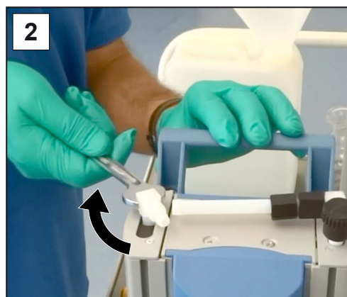
2. Turn the elbow union a quarter turn to the side; open-end wrench SW14.
