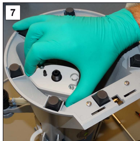
7. Pull out the VACUU-BUS plug downwards and remove the sensor.
