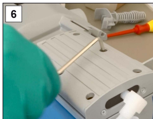
6. Unscrew the screw connections from the housing cover; Allen key 4.
