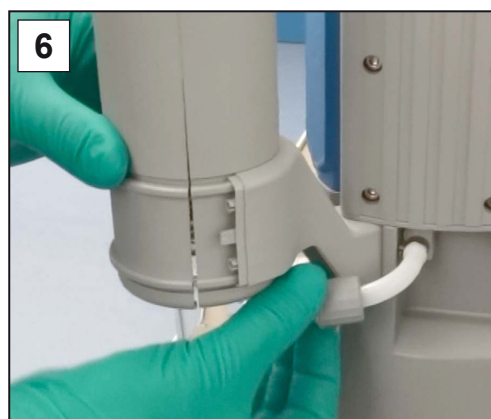
6. Attach the molded hose and tighten the knurled nut hand-tight.
