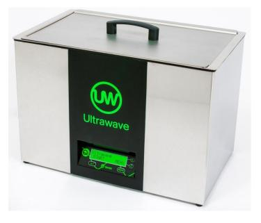
The **Qi-400** is a 30Litre ultrasonic cleaner with a menu driven, LCD control panel. This allows simple adjustment of cycle time (0 to 99mins or infinity mode), temperature (ambient to 80°C), ultrasonic power and frequency mode for precise and accurate processing.
